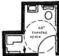
EXAMPLES OF ADAPTABLE BATHROOM LAYOUTS
