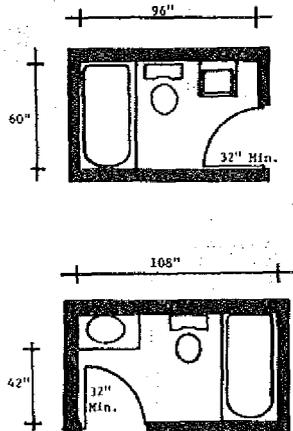
These examples may be modified for accessibility by using outward swinging doors or pocket sliding doors.
