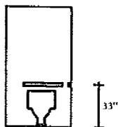
It is recommended that grab bars be from 30 to 42 inches in length and located no more than 12 inches from the back wall.
