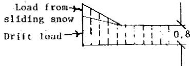
Design lower roof for loads applicable to multi-level roofs plus a portion of the sliding snow from the upper roof
