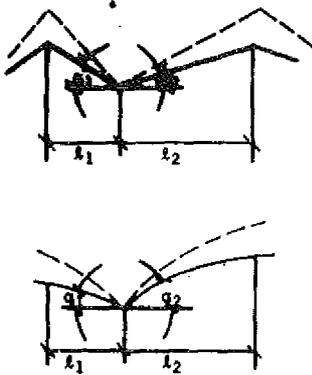
Valley areas of two-span and multiple series sloped or curved roofs
