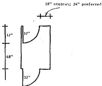
Doors in series should be hinged on the same side and should swing in the same direction. A minimum of 18 inches of clear space should be provided on the door knob side of the door. The length of the vestibule should be a minimum of 48 inches plus the width of the door in the open position (i.e., 32-inch door plus 48 inches length equals 80 inches overall length of vestibule).
