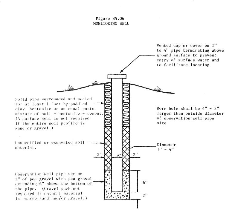
a. Except as provided in subpar. b., monitoring wells shall extend at least 3 feet below an expected depth of a system.
