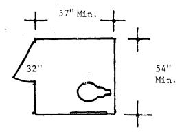
The door of the 54" x 57" water closet compartment having a frontal approach should not align with the placement of the water closet. This compartment configuration if preferred by the physically disabled.
