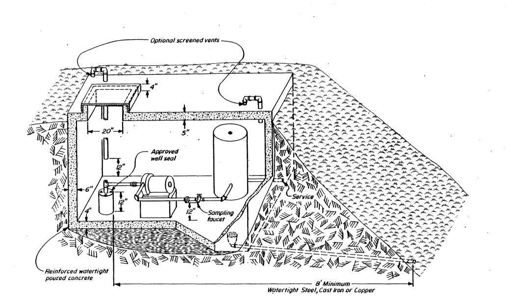
Figure 45. Minimum requirements for approved new well pits.
