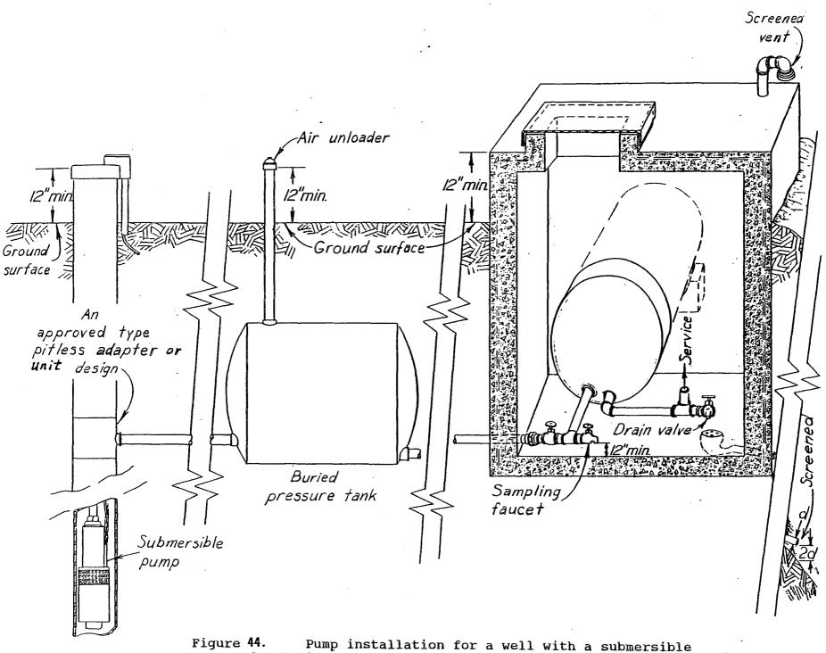
pump and a buried pressure tank less than 1,000 gallons, middle drawing, or greater than 1,000 gallons, at right.
