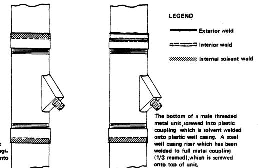
A male threaded metal unit screwed into plastic couplings, which are solvent welded onto plastic well casings.
