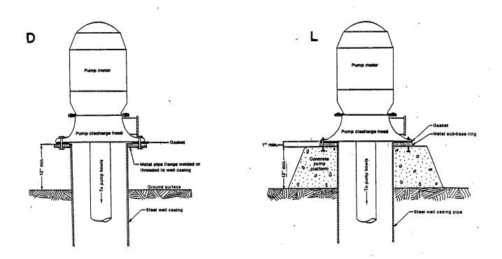
Figure 38. Pump installations for high capacity wells with lineshaft turbine pumps.
