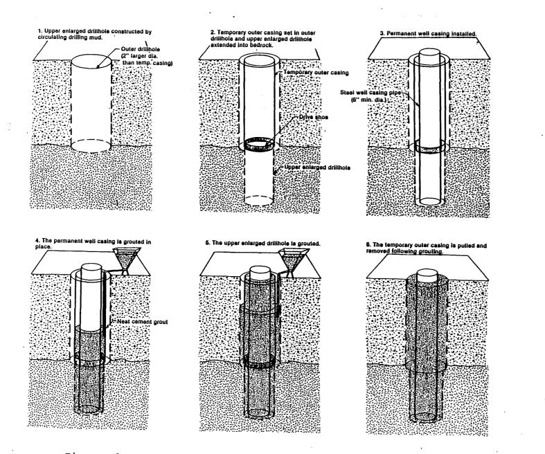
Figure 2. Required rotary method for constructing and sealing upper enlarged drillholes to enable the setting and removal of a temporary outer casing in bedrock wells overlain by unconsolidated caving material.
