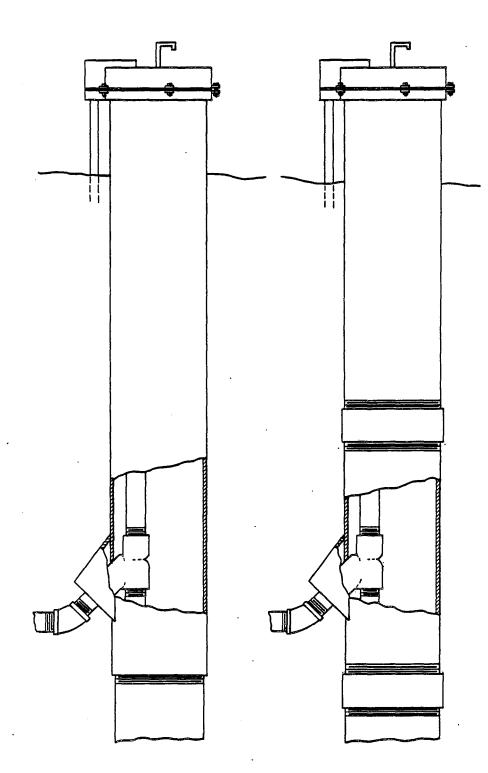
Figure 27. Non-spool type pitless units. (For acceptable procedures for connection of the units to the well casing pipe see s. NR 112.31(3)).
