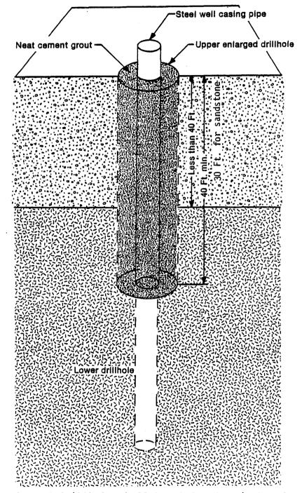
The upper enlarged drillhole shall be at least 2 inches larger in diameter than the nominal well casing pipe diameter for well casing pipe with welded joints. For threaded and coupled well casing pipe, the diameter shall be at least 4 inches larger than the nominal well casing pipe diameter. Figure 62. Line E. Rotary methods for low capacity\* and nonpotable high capacity wells in all types of bedrock with less than 40 feet of overlying non-caving material.
