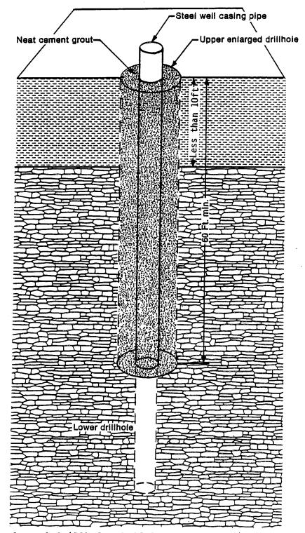
The upper enlarged drillhole shall be at least 2 inches larger in diameter than the nominal well casing pipe diameter for well casing pipe with welded joints. For threaded and coupled well casing pipe, the diameter shall be at least 4 inches larger than the nominal well casing pipe diameter.
