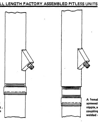
A female threaded metal unit screwed onto threaded steel pipe nipple, which is screwed into plastic coupling that has been solvent welded onto plastic well casing.
