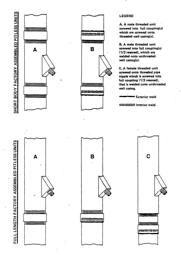
Figure 30. Pitless unit connections for wells with steel well casing pipe. NOTE: A well casing pipe nipple,  $\frac{1}{2}$  threaded  $-\frac{1}{2}$  beveled may be used in lieu of a full pipe coupling.
