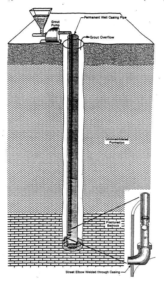
Figure 18. Street elbow method for neat cement grouting.
