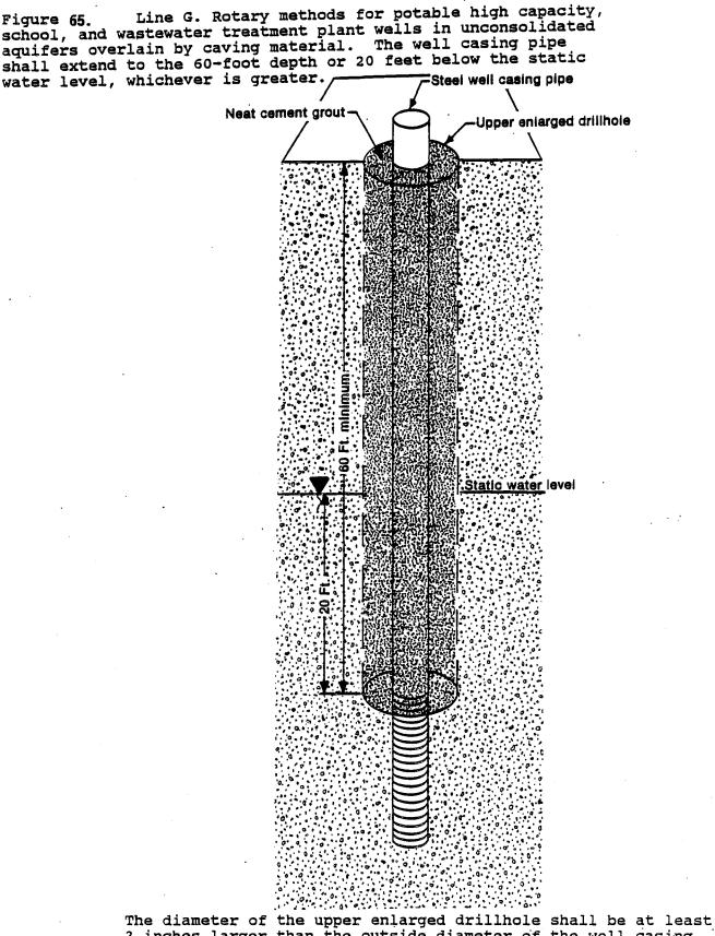
The diameter of the upper enlarged drillhole shall be at least 3 inches larger than the outside diameter of the well casing pipe or well casing pipe couplings, if used.
