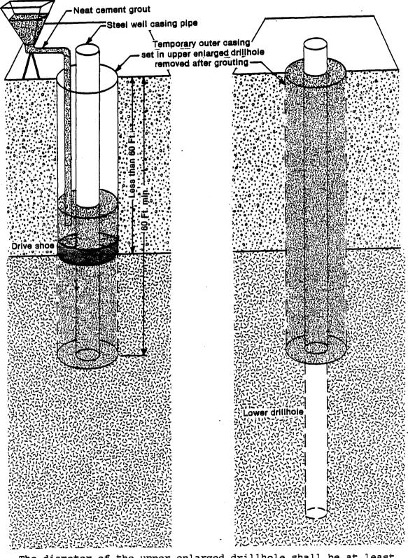
Figure 73. Line K. Rotary methods for potable high capacity, school, and wastewater treatment plant wells in all types of bedrock with less than 60 feet of overlying caving material.
