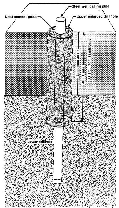
The upper enlarged drillhole shall be at least 2 inches larger in diameter than the nominal well casing pipe diameter for well casing pipe with welded joints. For threaded and coupled well casing pipe, the diameter shall be at least 4 inches larger than the nominal well casing pipe diameter. Figure 63. Line F. Rotary and percussion methods for low capacity\* and nonpotable high capacity wells in limestone and dolomite with less than 20 feet of overlying material.
