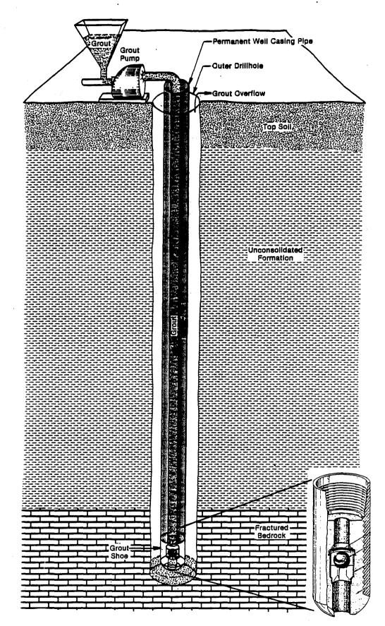
Figure 13. Grout (float) shoe-pumped method for neat cement grouting.
