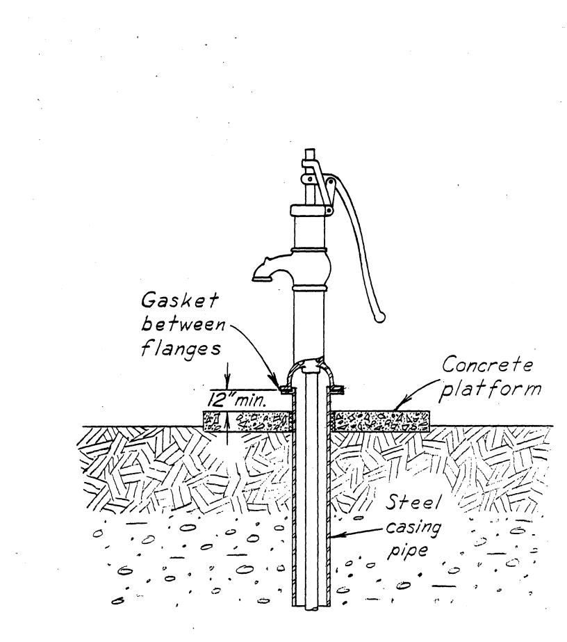
Figure 40. Pump installation for wells with hand pumps.
