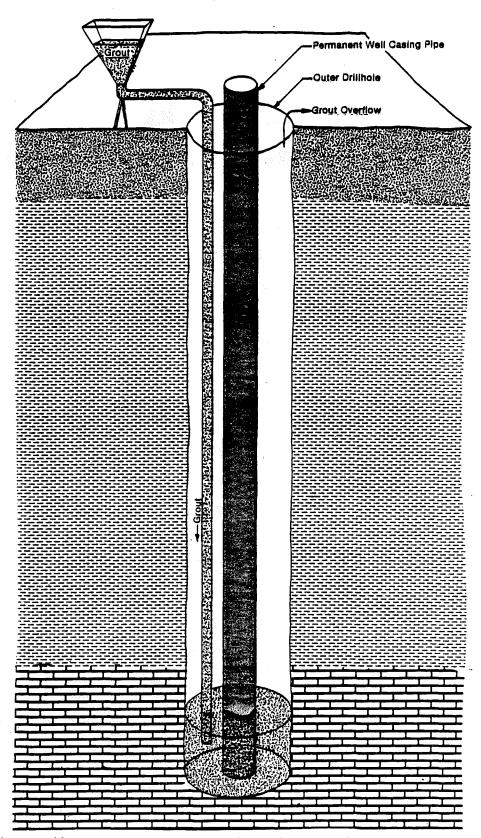
Conductor (tremie) pipe - gravity method
