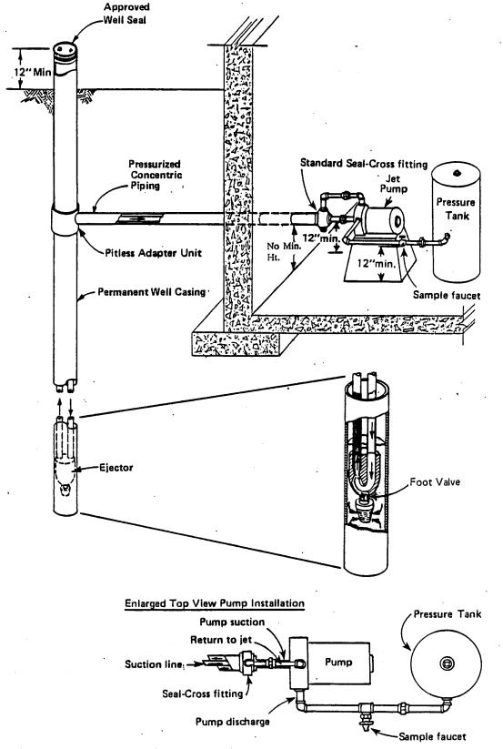
Figure 35. Pump installation for a deep well jet pump assembly with a pressure conduit having a concentric piping arrangement. A pressure (box) elbow may be used to extend the pressurized conduit to a point above the basement floor. The pressure (box) elbow may be buried.
