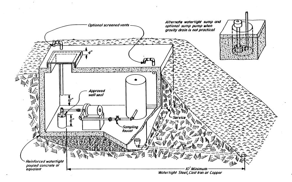
Figure 47. Minimum requirements for existing well pits.
