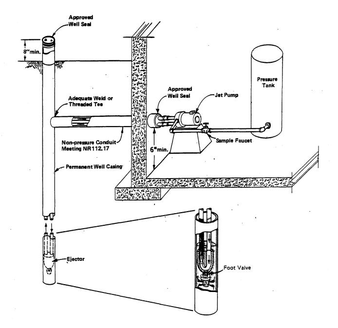
Figure 50. Pump installation for an existing well with a deep well jet pump assembly and a non-pressure conduit.
