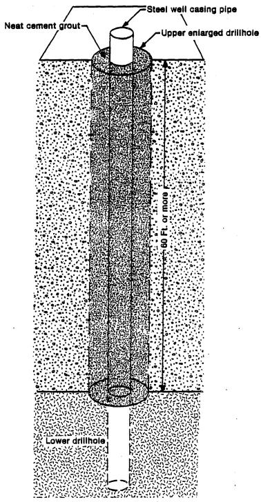
The diameter of the upper enlarged drillhole shall be at least 3 inches larger than the outside diameter of the well casing pipe or well casing pipe couplings, if used. The diameter of the well casing pipe and lower drillhole shall be at least 6 inches.
