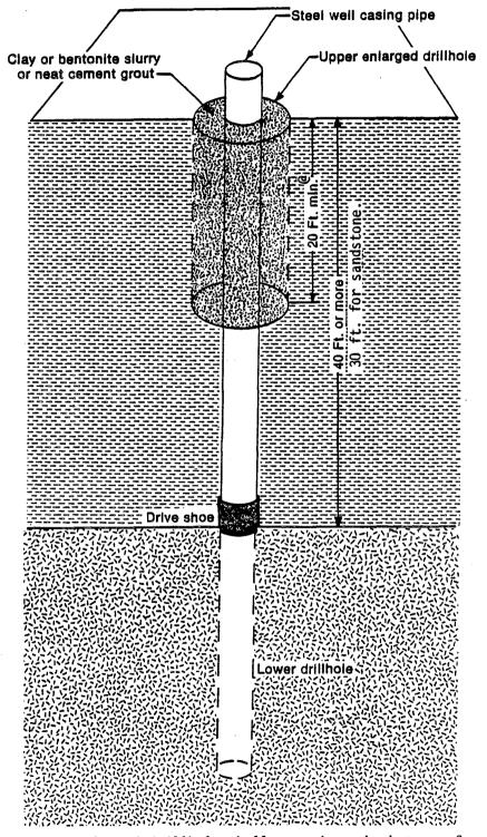
@ The upper enlarged drillhole shall extend to the bottom of any non-caving material or to the 20-foot depth, whichever is the lesser. As an alternative to constructing an upper enlarged drillhole, granular (8-mesh) bentonite may be mounded surrounding the well casing pipe during driving. Figure 58. Line D. Rotary methods for low capacity\* and nonpotable high capacity wells in all types of bedrock with at least 40 feet of overlying non-caving material.
