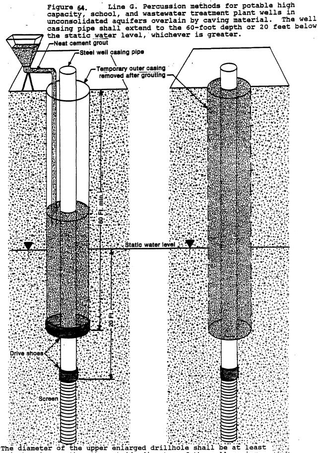
3 inches larger than the outside diameter of the well casing pipe or well casing pipe couplings, if used. The diameter of the well casing pipe and lower drillhole shall be at least 6 inches.
