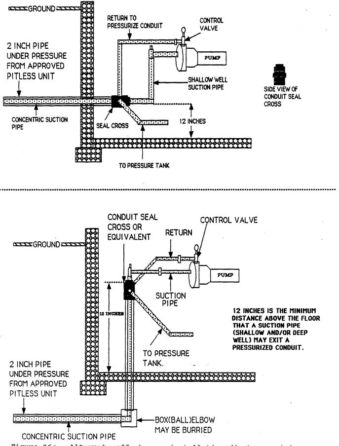
Figure 36c. Alternate offset pump installation discharge piping using a buried box (ball) elbow and seal cross fitting. Figure prepared by T. Roos.
