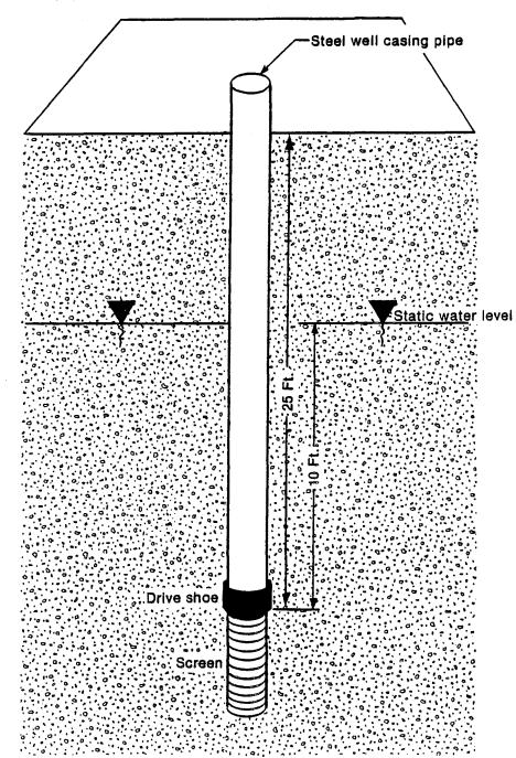
The well casing pipe may be driven from the ground surface.
