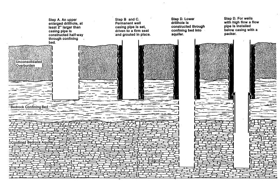
Figure 10. (c)2. Rotary method flowing well construction - confined bedrock aquifer more than 40<sup>@</sup>feet below the ground surface with a bedrock confining bed.
