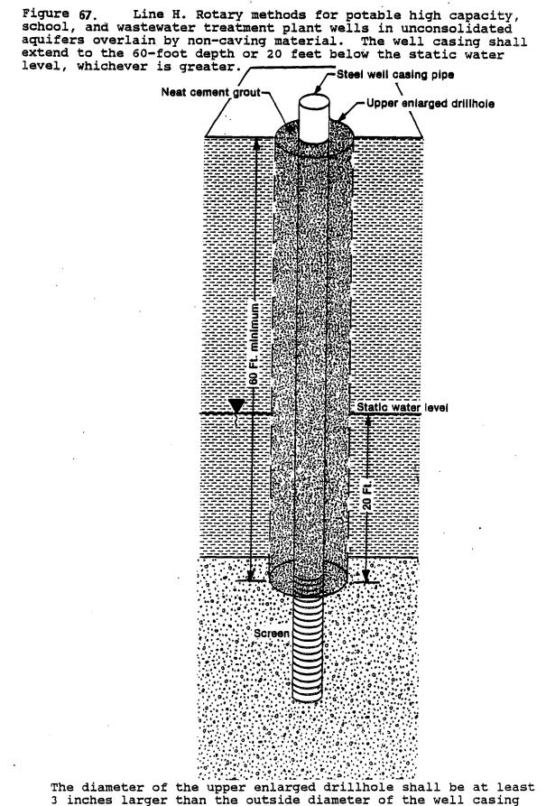
pipe or well casing pipe couplings, if used. During construction the upper enlarged drillhole shall be
