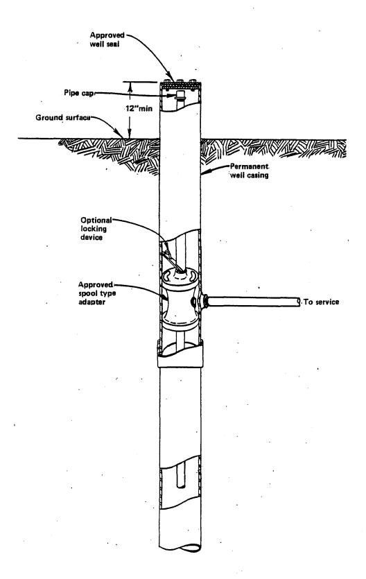
Figure 26. Factory-assembled spool pitless unit installation. (For acceptable procedures for connection of the unit to the well casing pipe see s. NR 112.31(3)).
