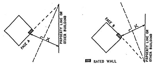
The following sketch shows setback measurements between intersecting or projected intersection of building faces.
