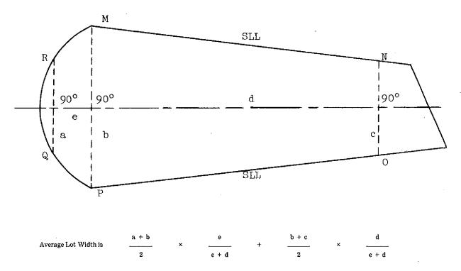
Area of MNOPQR equals Minimum Lot Area and line d bisects angle formed by lines MN and OP extended. d is the perpendicular distance between b and c. e is the perpendicular distance between lines a and b.
