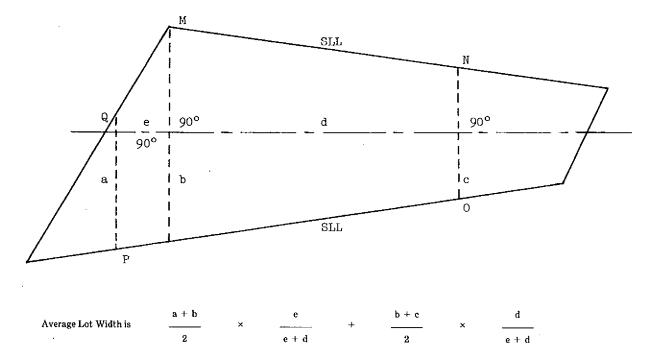
Area of MNOPQ equals Minimum Lot Area and line d bisects angle formed by lines MN and OP extended. d is the perpendicular distance between lines b and c. e is the perpendicular distance between lines a and b.
