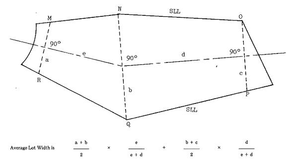
Area of MNOPQR equals Minimum Lot Area, line e bisects angle formed by MN and QR extended and line d bisects angle formed by NO and PQ extended. d is the perpendicular distance between b and c. e is the perpendicular distance between a and b.
