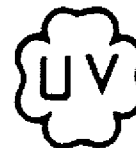
FIG. UG-129.1 OFFICIAL SYMBOL FOR STAMP TO DENOTE THE AMERICAN SOCIETY OF MECHANICAL ENGINEERS' STANDARD FOR PRESSURE RELIEF VALVES
