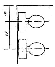
Figure 84.20-1. Spacing between water closets.
