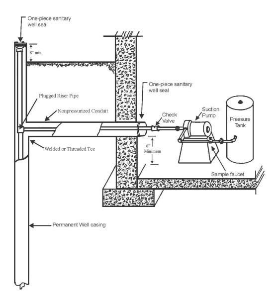
Figure 14. Pump installation for a deep well jet pump assembly and a nonpressurized conduit installed prior to Febuary 1, 1991
