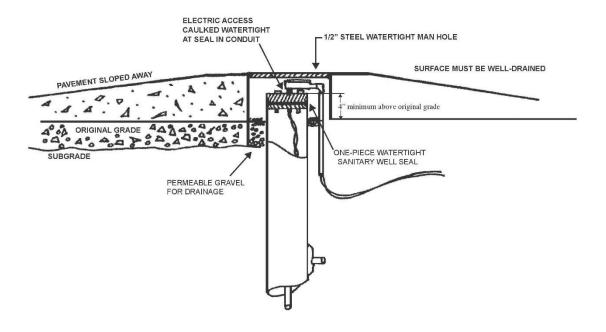
Figure 11. Well pits - Minimum requirements for pits installed on or before April 10, 1953.
