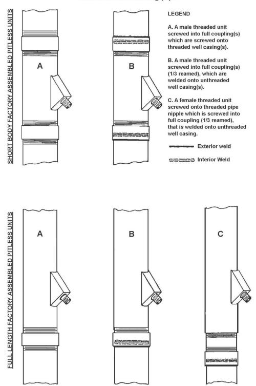
Figure 2. Pitless unit connections for wells with thermoplastic well casing pipe.
