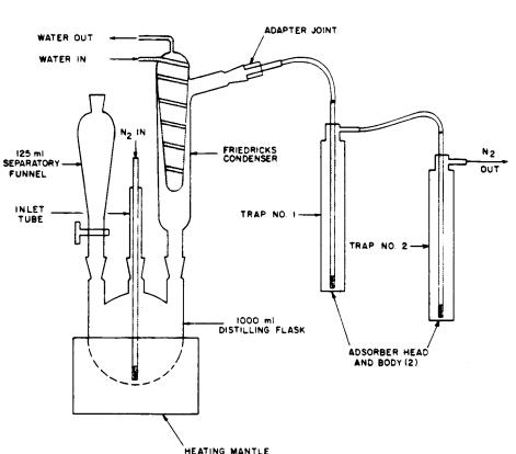
FIGURE 1 EQUIPMENT ASSEMBLY
