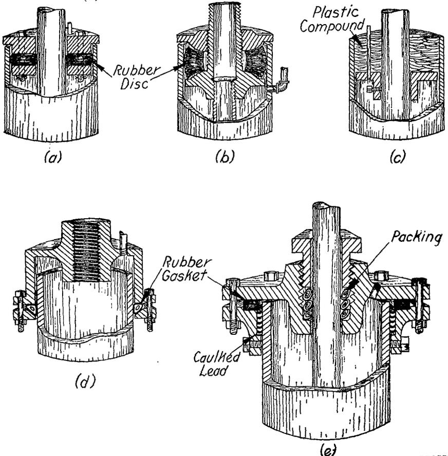
Figure 11. Types of Well Seals. (a) and (b): Seals using inside compressed rubber. (c) using inside plastic compound. (d) using outside compressed rubber gasket. (e) using caulked lead, compressed rubber and packing. See Wis. Adm. Code section RD 12.09 (3).
