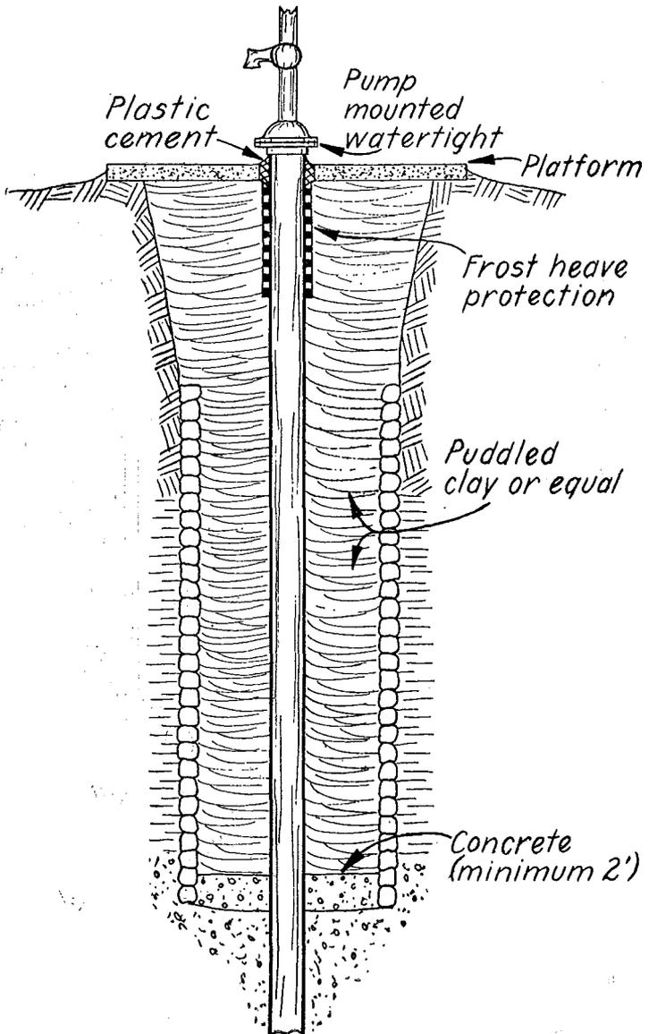
Figure 9. Drilled Well Constructed in Existing Dug Well. See Wis. Adm. Code section RD 12.05 (7).
