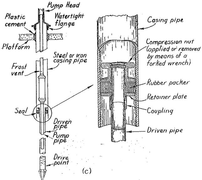
Figure 7. Driven Point Well Construction. Illustration (c) shows suitable method of returning frost drain water to well when impervious soil is present. See Wis. Adm. Code section RD 12.05 (5).
