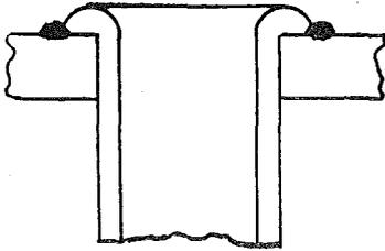
Seal welding shall be applied in one light layer if practicable but not more than two layers shall be used—Throat dimension shall not exceed  $5/16$ ".
