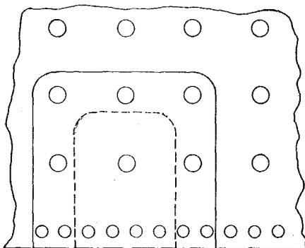
Patches shall be of material equal to the original in quality and thickness.
