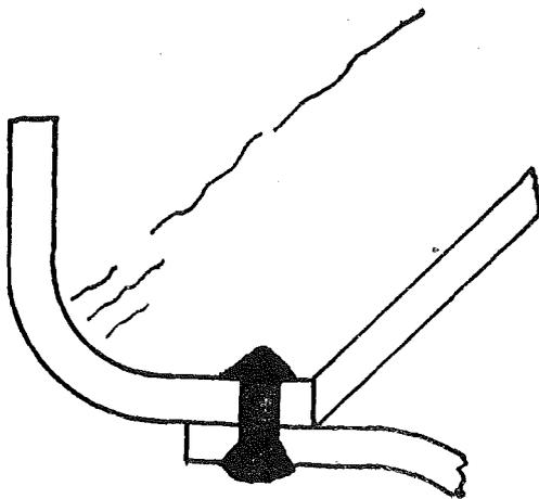
Field repair of cracks at knuckle or turn of flange of furnace opening is difficult. It is recommended that this repair be made in a well equipped shop.
