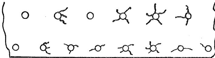
Multiple or star cracks radiating from staybolts or rivet holes shall not be repaired by welding.
