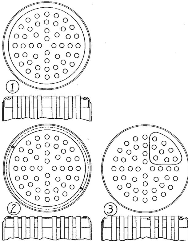
**1. Flush Butt Welded Head**
