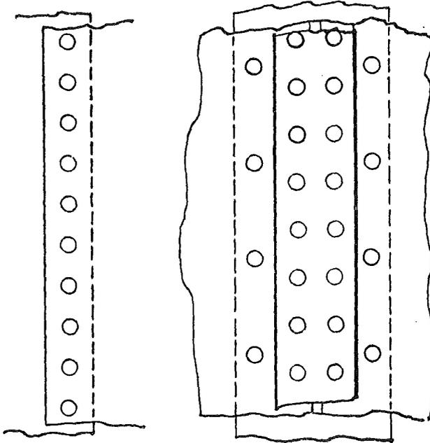
**Caution.**—Seal welding shall not be applied if cracks are present in riveted areas.
