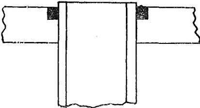
In water tube boilers, tubes may be seal welded on inside or outside of tube sheet.
