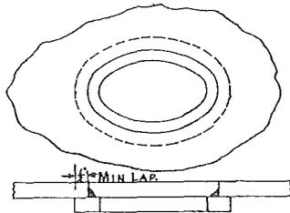
Plate lap should not be less than  $\frac{1}{2}$ ".
