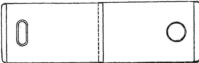
Before any effort is made to patch a bagged or deformed area the original shape or curvature shall be restored as far as possible. Patch shall be rolled or pressed to proper shape or curvature. Edges shall align without overlap.
