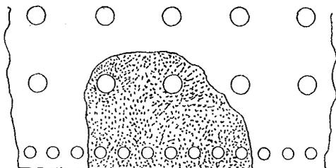
If corroded area includes rivets or staybolts, these shall be removed before welding is applied.
