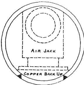
When practicable, a removable copper backup recessed as shown to provide complete weld penetration through the tube wall and held in place by a removable air jack shall be used during the welding operation.
