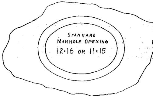
A badly corroded manhole flange may be repaired by cutting out flanged section and inserting a ring type frame as shown. Dimensions shall comply with requirements of sections Ind 41.50 and Ind 41.51 of this code.
