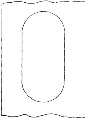
This type of patch may be used if necessary to seal a hole cut in a water wall tube to provide access for welding the back side of a circum. joint or to replace a small sharp bag.
