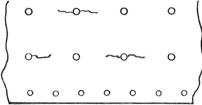
**Caution:** Before attempting repairs to cracks of this type the inner surface of the plate shall be carefully examined for possible excessive corrosion or grooving.
