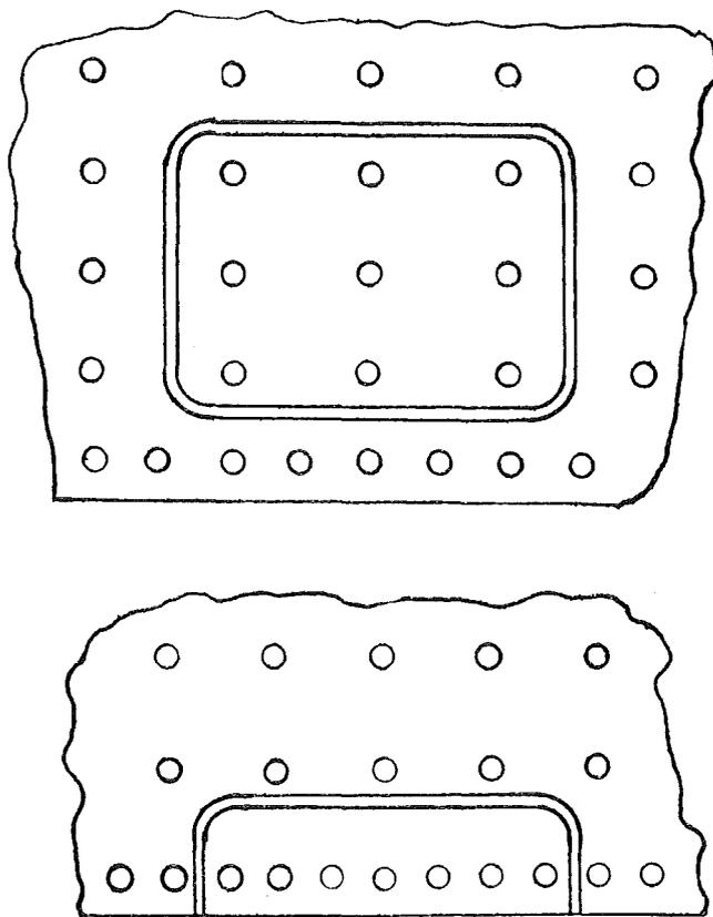
Patches shall be of material equal to the original in quality and thickness.
