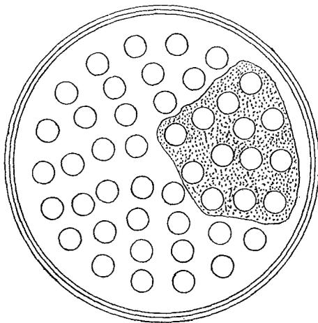
Corroded areas of tube sheets may be built up by welding where tubes act as stays.
