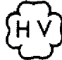
FIG. HG-402 OFFICIAL SYMBOL FOR STAMP TO DENOTE THE AMERICAN SOCIETY OF MECHANICAL ENGINEERS' STANDARD
