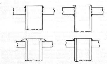
Tubes may be seal welded provided the ends of the tubes have sufficient wall thickness to prevent burn through. Seal welding should be applied with a maximum of three light layers in lieu of one or two heavy layers.
