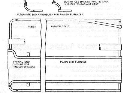
Longitudinal seam in furnace double butt-welded and thermally stress-relieved. For repair, final joint to each head may be stress-relieved by peening. Furnace may be welded into a riveted boiler by using adaptable end closures. Ringed furnace shall be thermally stress-relieved after longitudinal seam and rings have been applied.
