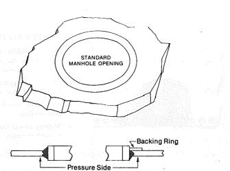
A badly wasted manhole flange may be removed and replaced with a ring-type frame as shown above. The requirements of 42.150 for flush patches shall be met. A full penetration weld is required. May either be double welded or welded from one side with or without a backing ring.
