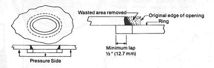
A badly wasted area around a handhole opening may be repaired by adding a ring as shown above on the inside of the object.
