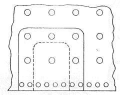
Patches shall be of material equal to the original in quality and thickness.
