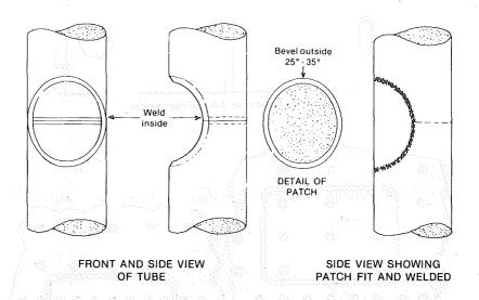
It may be necessary to weld a flush patch on a tube, since in some situations, accessibility around the complete circumference of the tube is restricted. Listed below are suggested methods for making window patches:
