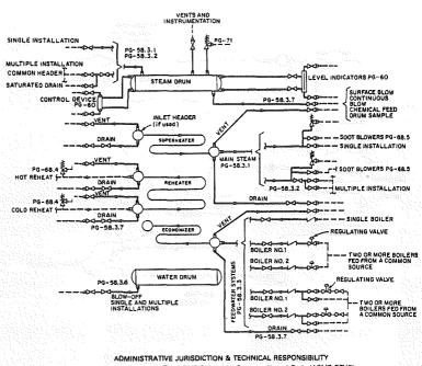
Boiler Proper — The ASME Boiler and Pressure Vessel Code (ASME BPVC)
