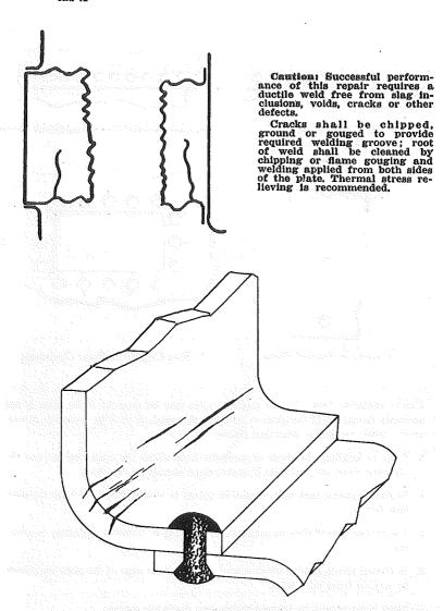
Cracks at the knuckle or at the turn of the flange of the furnace opening require immediate replacement of the affected area. If repairs are attempted, specific approval of the department is required.
