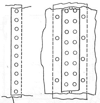
Caution.—Seal welding shall not be applied if cracks are present in riveted area.
