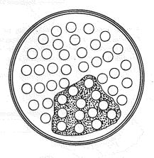
Wasted areas in stayed and unstayed surfaces may be built up by welding provided that in the judgment of the Inspector the strength of the structure will not be impaired. Where extensive weld build-up is employed, the Inspector may require an appropriate method of NDE for the complete surface of the repair.
