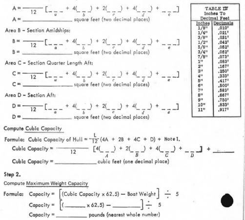
Note 1: The volume of integral structure aft of the transom below the static float line may be added to the claculated cubic capacity.
