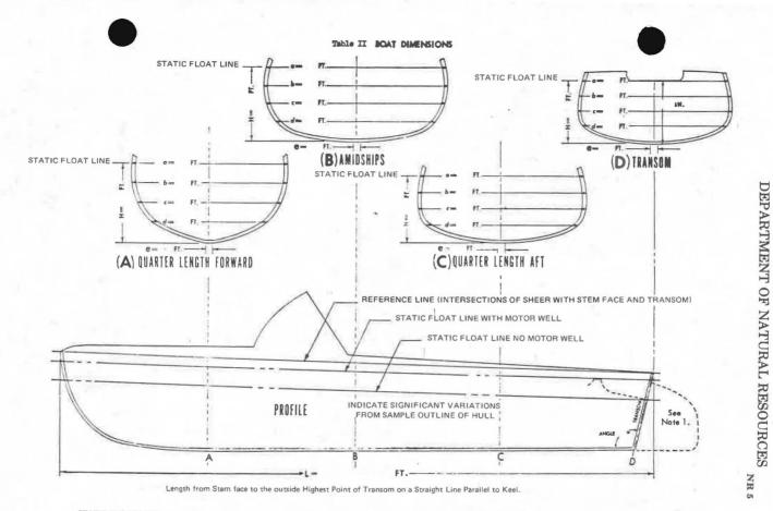
STATIC FLOAT LINE passes through the point of major leakage and is parallel with a line connecting the intersections of the sheer with the forward face of the stem and the sheer with the afterface of the transom.
