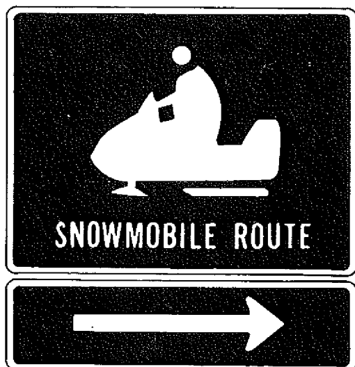
GREEN-REFLECTORIZED BACKGROUND WITH WHITE-REFLECTORIZED LETTERS AND SYMBOLS
