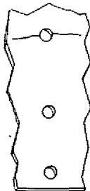
Cracks in Stayed Plates
