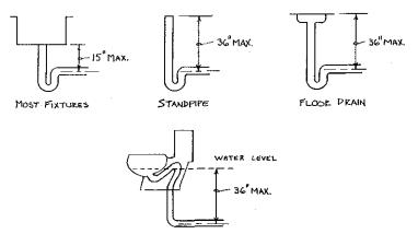
VERTICAL DISTANCE BETWEEN FIXTURE DRAIN OUTLET AND TEAP
