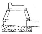
STANDARD STORM WATER INLET (MASONRY)
