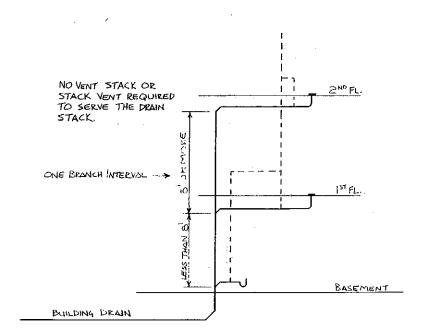
A-82.31 (4) (b) Installation of vent stack and stack vent.
