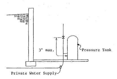
A-82.40 (5) (a) Storage tank and piping insulation. The following is a reprint of section ILHR 63.63.
