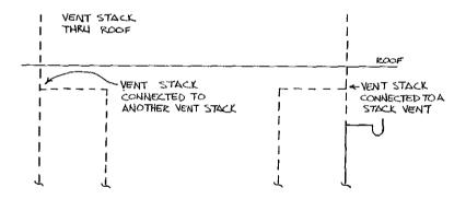
A-82.31 (4) (b) Installation of vent stack and stack vent.
