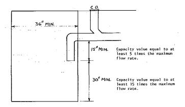
CAL WASH INTERCEPTOR WITH CAST IRON INVERT INSIDE OF BASIN
