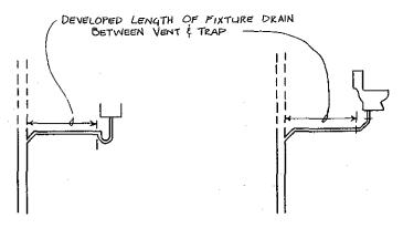
WHERE TRAP IS NOT AN INTEGRAL PART OF THE FIXTURE
