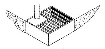
FLOOR SINK WITH GRATE OPENING FOIL AIR GAP
