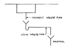
A-82.33 (8) (a) Waste sinks and standpipes.
