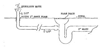
3. Battery assemblies. A battery assembly of not more than 3 sterilizer wastes may drain to one trap, provided the trap and waste are sized according to the combined fixture unit rating; the trap is located immediately below one of the indirect waste connections; the developed distance
