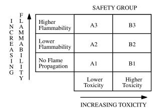
Note: Single-component refrigerants and azeotropic blends are classified by the American Society of Heating, Refrigerating and Air-Conditioning Engineers (ASH-RAE) and specified in ASHRAE Standard 34 along with the criteria for classification. The safety group classifications shown in Table 45.17–1 originate in ASHRAE Standard 34. Additional refrigerants are included in ASHRAE Standard 34. As new data becomes available, refrigerant classifications are subject to change in ASHRAE Standard 34.
