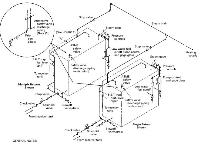
(a) Return connections shown for a multiple boiler installation may not always insure that the system will operate properly. In order to maintain proper water levels in multiple boiler installations, it may be necessary to install supplementary controls or suitable devices. (b) Plumbing codes may require the installation of a reduced pressure principle backflow preventer on a boiler when the makeup water source is from a potable water supply.
