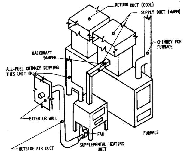
(9) **SUPPLY DUCTS.** Supply ducts connected to solid-fuel-burning appliances shall have the following minimum clearances to combustibles:
