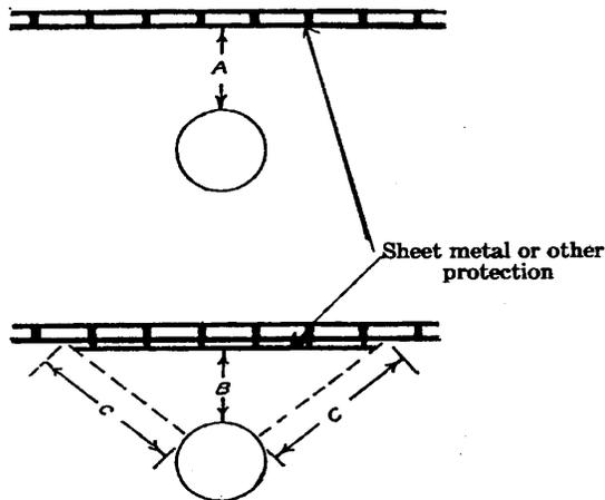
“A” Equals the required clearance with no protection, specified in s. SPS 323.045 (4) (b).
