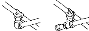
Figure 5-8.3(a) Replacement of elbow at end of cross main with a flushing connection consisting of a 2-in. nipple and cap.
