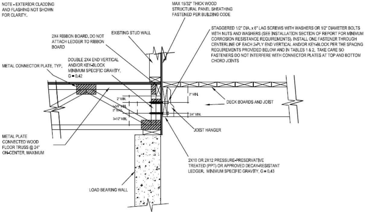
**PLACEMENT OF LAG SCREWS AND BOLTS IN LEDGER**
