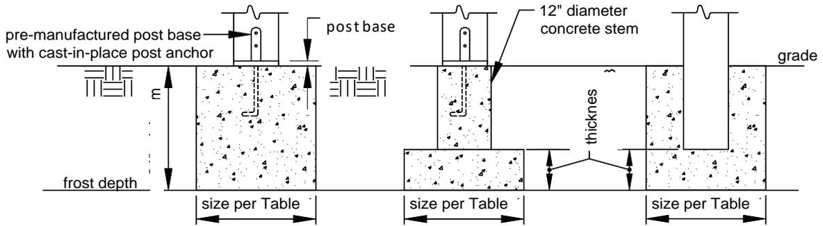
**SECTION 3: POSTS AND POST-TO-BEAM CONNECTIONS**
