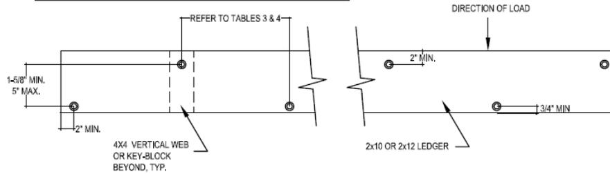
**KEY-BLOCK DETAIL FOR LEDGER ATTACHED TO SIDE OF FLOOR LADDER FRAME**
