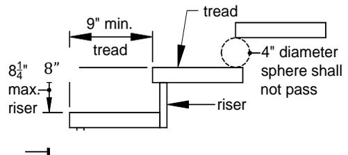
4. Within a stairway flight, the largest tread depth may not exceed the smallest tread depth by more than 3/8 inch, and the largest riser height may not exceed the smallest riser height by more than 3/8 inch.
