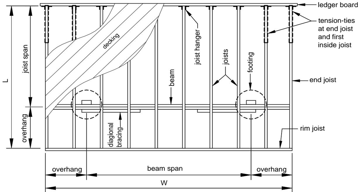
**Decking:**     2x4     2x6     five-quarter board     wood-plastic composite (per ASTM D 7032)
