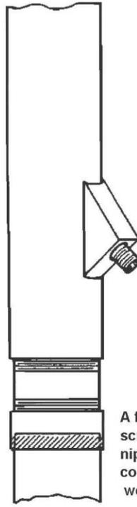
A female threaded metal unit screwed onto threaded steel pipe nipple, which is screwed into plastic coupling that has been solvent welded onto plastic well casing.
