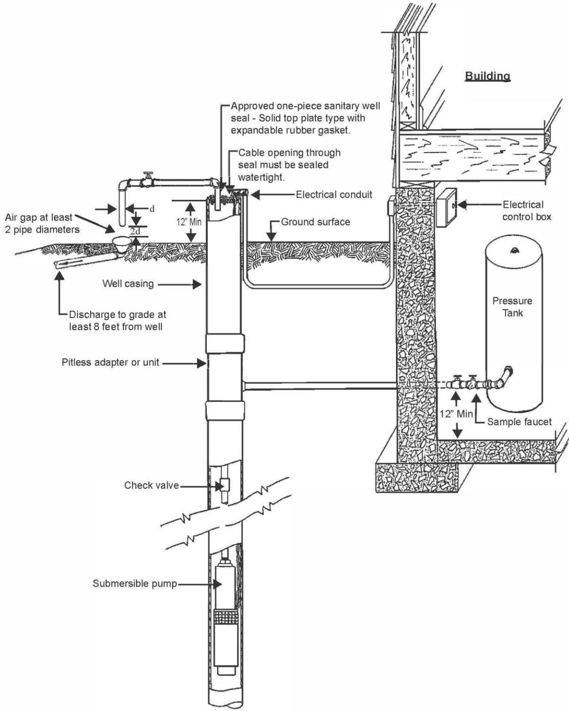
Figure 5. Flowing well - surge tank installation.
