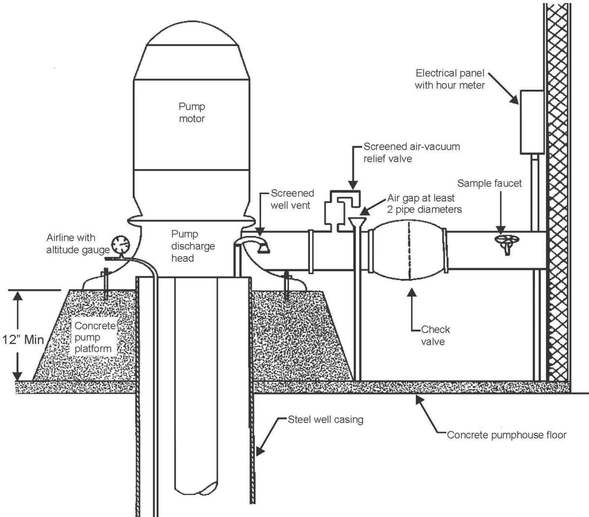
**Figure 4. Flowing well - Overflow piping arrangement with a submersible pump.**
