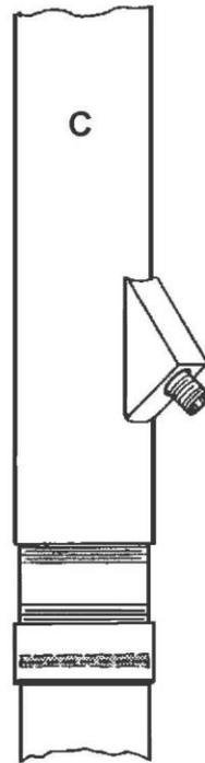
**Figure 2. Pitless unit connections for wells with thermoplastic well casing pipe.**
