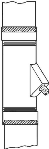
A male threaded metal unit screwed into plastic couplings, which are solvent welded onto plastic well casings.
