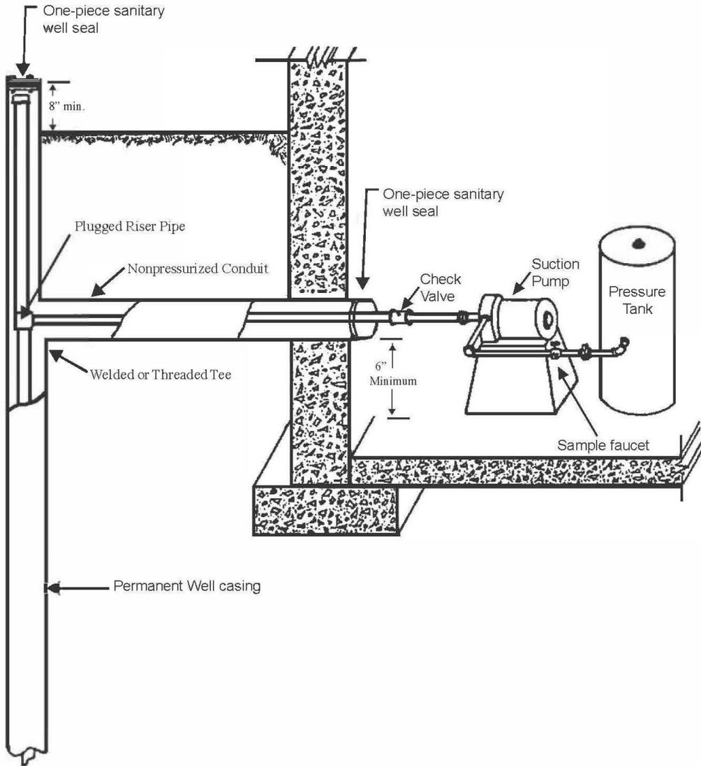
**Figure 13. Pump installation for a deep well jet pump assembly and a nonpressurized conduit installed prior to February 1, 1991**
