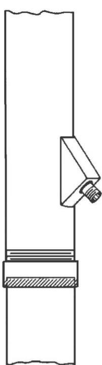
A male threaded metal unit screwed into plastic coupling, which is solvent welded onto plastic well casing.
