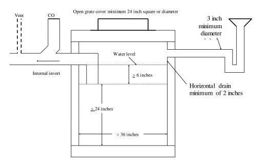
A-82.34 (4)-4. FIXTURES WITHOUT TRAPS DISCHARGING TO CATCH BASIN.
