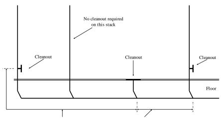
Developed length of drain piping between cleanouts not exceeding 40 feet for 2 inch ID or less, 75 feet for pipe with an ID of greater than 2 inches
