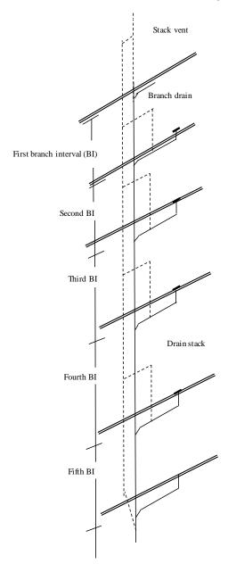
A-82.31 (4)-2. INSTALLATION OF VENT STACK AND STACK VENT.
