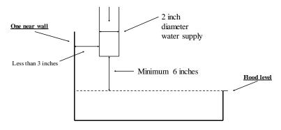
If distance is 3 times or greater than the diameter of water supply (2 inch), then the air-gap is 2 times the diameter of the water supply,
