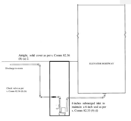
ELEVATOR DRAIN DISCHARGE - STORM DRAIN CONNECTION
