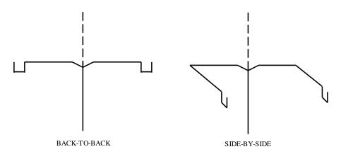
$A\hbox{-82.31 (11) (b) COMMON VENTS, HORIZONTAL DRAINS.}$
