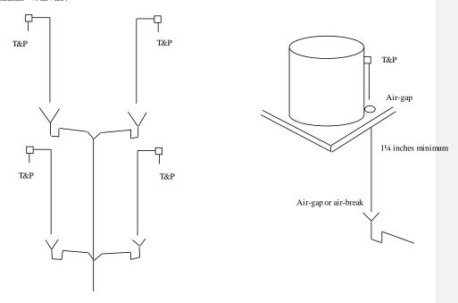
A-82.33 (9) (c) COMMERCIAL GRAVITY DISCHARGE-TYPE CLOTHES WASHERS.
