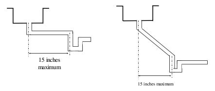
HORIZONTAL DISTANCE BETWEEN FIXTURE DRAIN OUTLET AND
