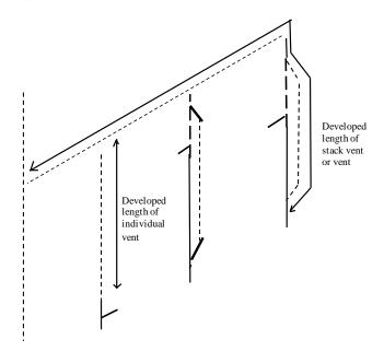
A-82.31 (14) (c) SIZING BRANCH VENTS SERVING A WET VENT.
