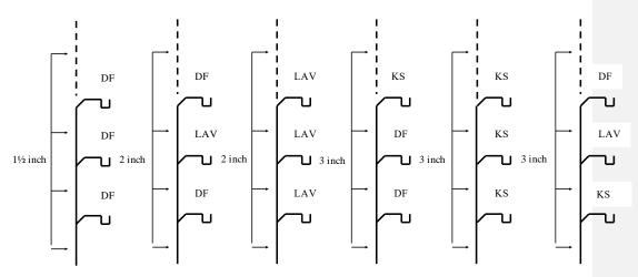
Most restrictive fixture determines stack size
