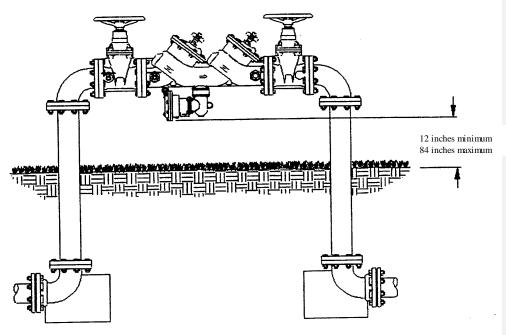
REDUCED PRESSURE ASSEMBLY OUTDOOR INSTALLATION
