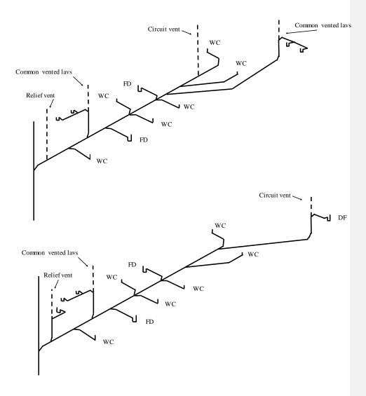
A-82.31 (11) (a) COMMON VENTS, VERTICAL, SERVING ANY TWO FIXTURES.
