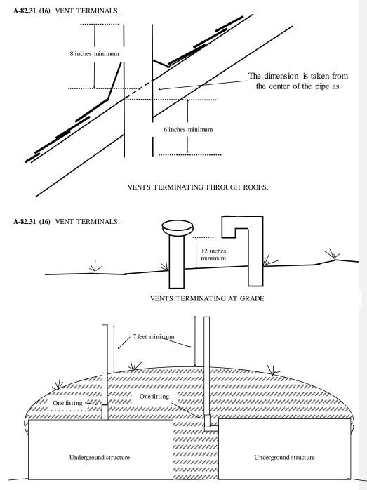
VENTS TERMINATING FOR UNDERGROUND STRUCTURES
