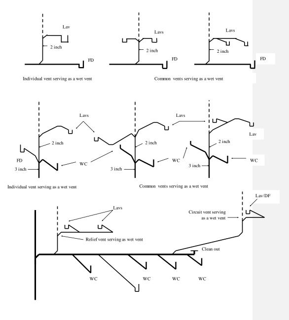
A-82.31 (14) (a) and (b) SIZING VENT STACKS AND STACK VENTS
