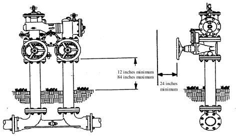
REDUCED PRESSURE ASSEMBLY OUTDOOR INSTALLATION
