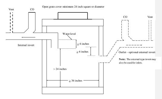
A-82.34 (4)-2. TRAPPED FIXTURES DISCHARGING TO CATCH BASIN.
