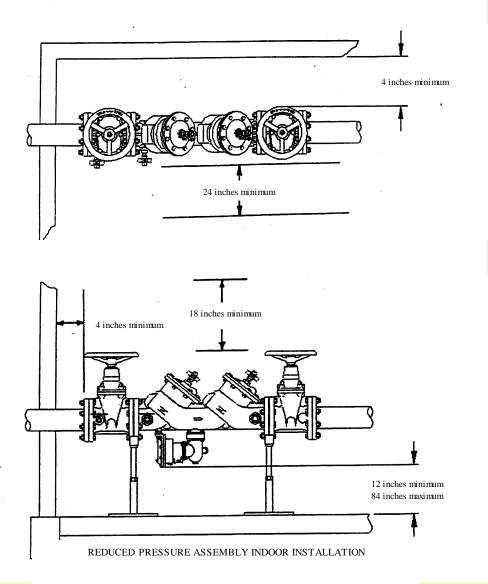
A-82.41 (5) (f)-2. CROSS CONNECTION CONTROL ASSEMBLY INSTALLATION.
