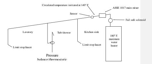
$\textbf{Option 5.} \ \ \text{Fail safe solenoid, combination pressure balanced/thermostatic tub/shower valve meeting ASSE 1016 and thermostatic mixer meeting ASSE 1016 at lavatory and kitchen sink faucets.$
