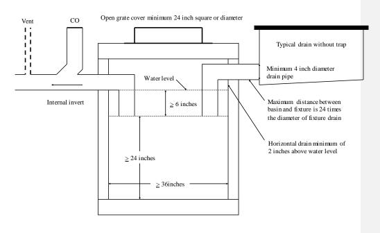
A-82.34 (4)-5. GARAGE CATCH BASIN WITH FIXTURES ON SEPARATE FLOOR LEVELS.
