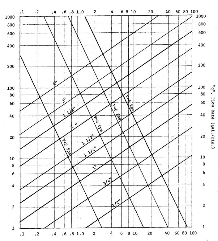
"p", Pressure Loss Due To Friction (psi/100 ft. of pipe)
