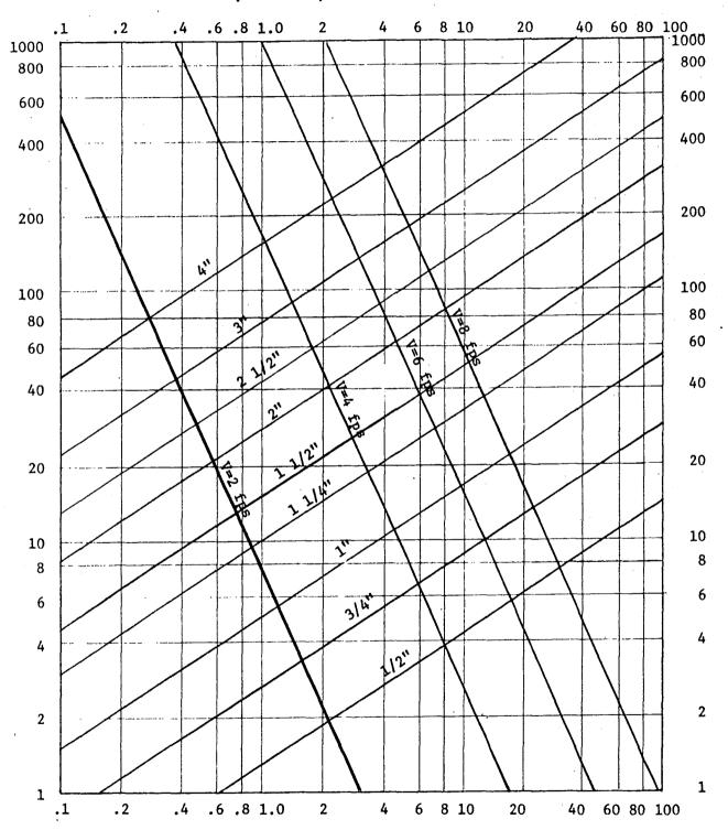
"p", Pressure Loss Due To Friction (psi/100 ft. of pipe)
