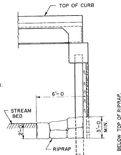
LONGITUDINAL SECTION WITHOUT BERM
