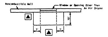
b. For second story windows, the transformer shall not be located less than 5' from any part of the window. See Figure PSC 317AB3b.
