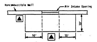
3.a. Padmounted oil-insulated transformers shall not be located within a zone extending 10' outward and 3' to either side of a building window or opening other than an air intake. See Figure PSC 114-317AB3a.
