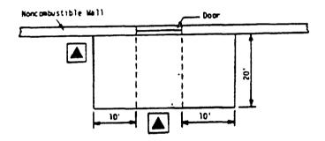
2. Padmounted oil-insulated transformers shall not be located within a zone extending 10' outward and 10' to either side of an air intake opening. Such transformers may be located within said zone beneath an air intake opening provided there is not less than 25 feet diagonal separation between the transformer and said opening. See Figure PSC 114-317AB2.
