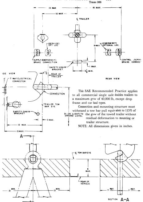
Clearance space shown must extend 7 in. above and 7 in. below the horizontal centerline of the drawbar eye as shown in Section A-A. NOTE: All dimensions given in inches.
