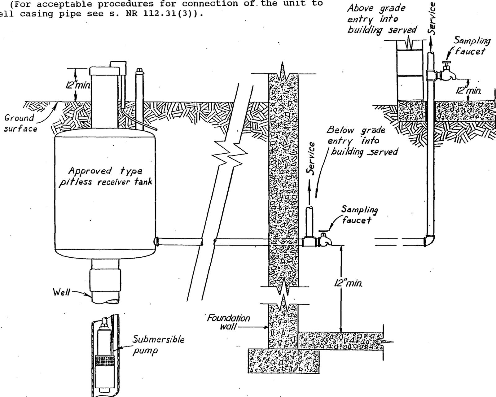
(4) HOLD-DOWN DEVICE. Well caps or seals may not be used as a hold-down device to prevent submersible pump discharge piping from coming off a pitless adapter or unit. A locking clamp or other similar approved device may be used to hold the submersible pump discharge pipe in place.
