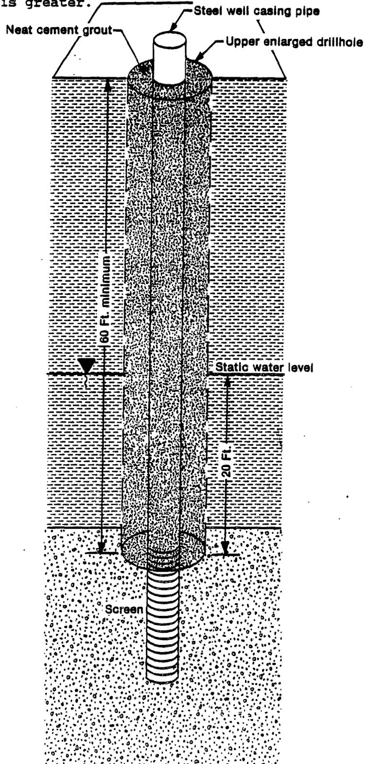
The diameter of the upper enlarged drillhole shall be at least 3 inches larger than the outside diameter of the well casing pipe or well casing pipe couplings, if used.
