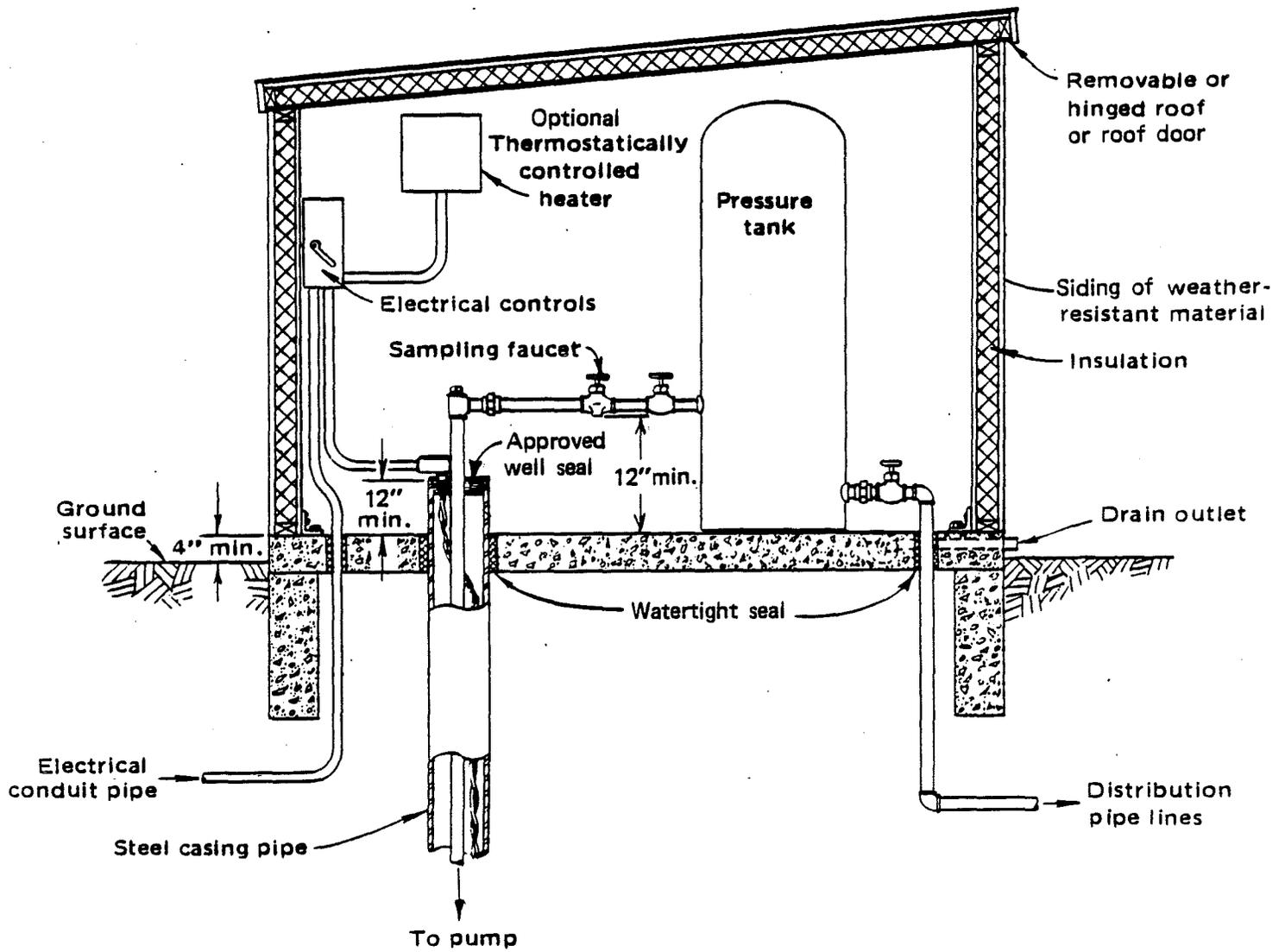
Figure 46. Pumphouse specifications.
