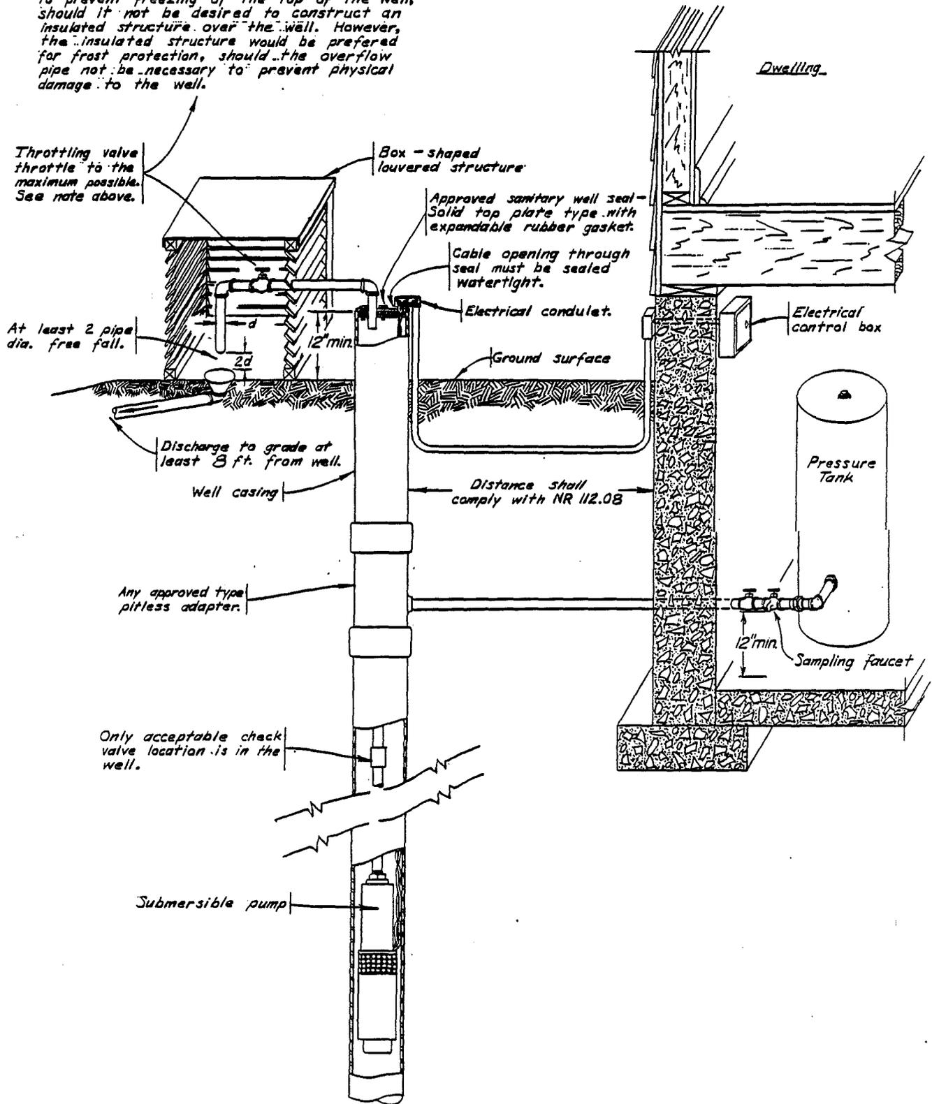
Figure 41. Overflow piping arrangement for a flowing well with a submersible pump.
