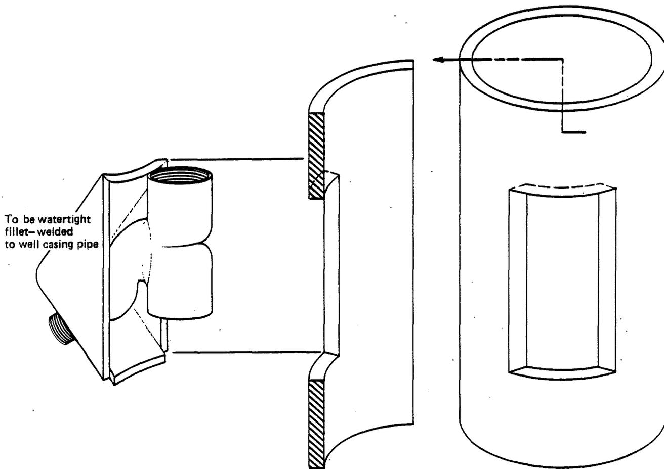
Figure 28. A weld-on pitless adapter.
