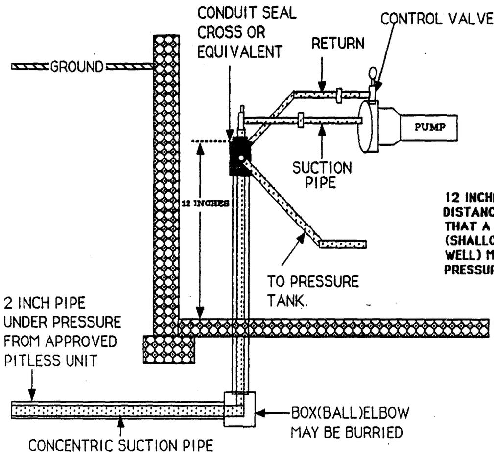
**12 INCHES IS THE MINIMUM DISTANCE ABOVE THE FLOOR THAT A SUCTION PIPE (SHALLOW AND/OR DEEP WELL) MAY EXIT A PRESSURIZED CONDUIT.**
