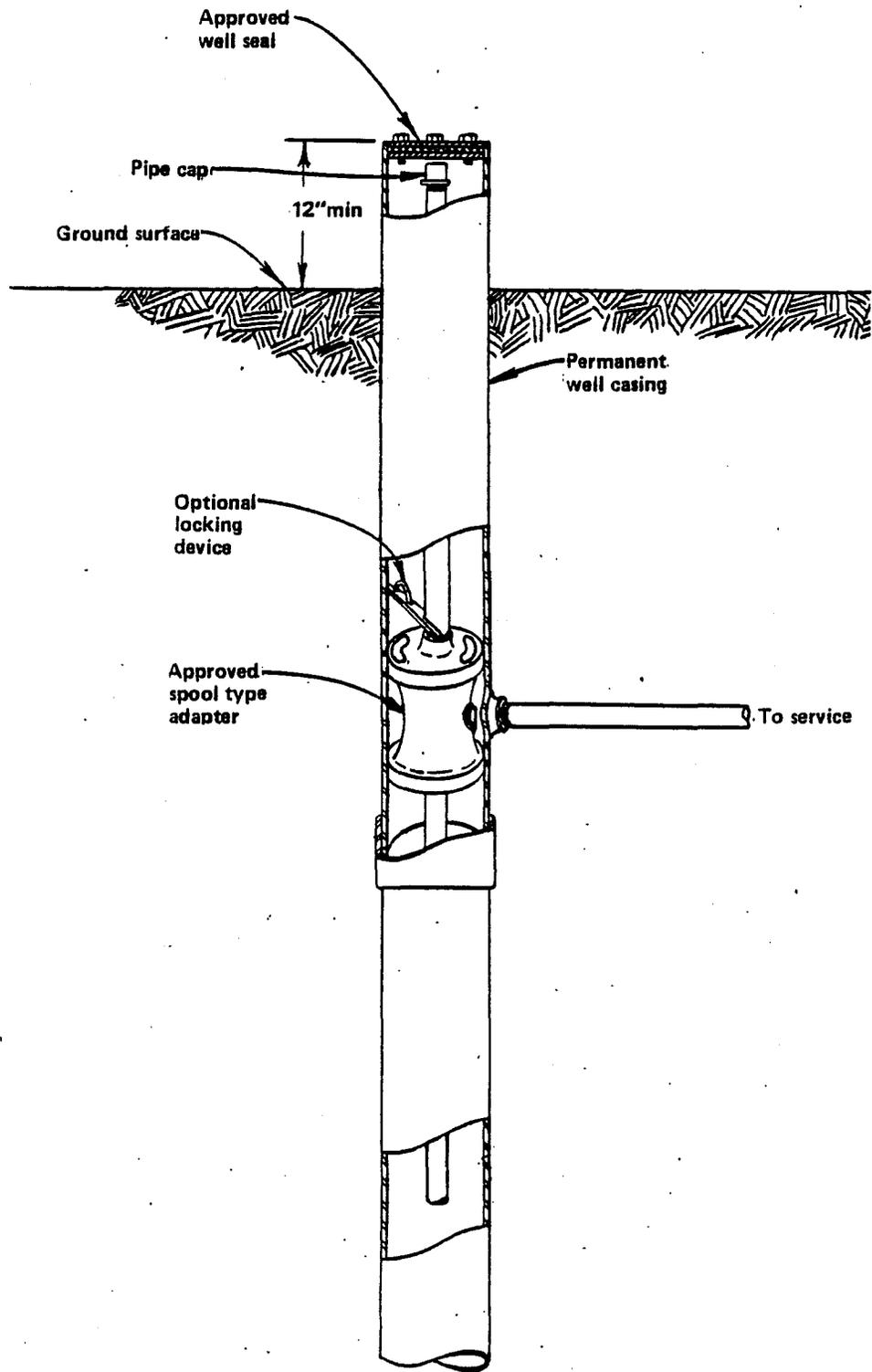
Figure 26. Factory-assembled spool pitless unit installation.
