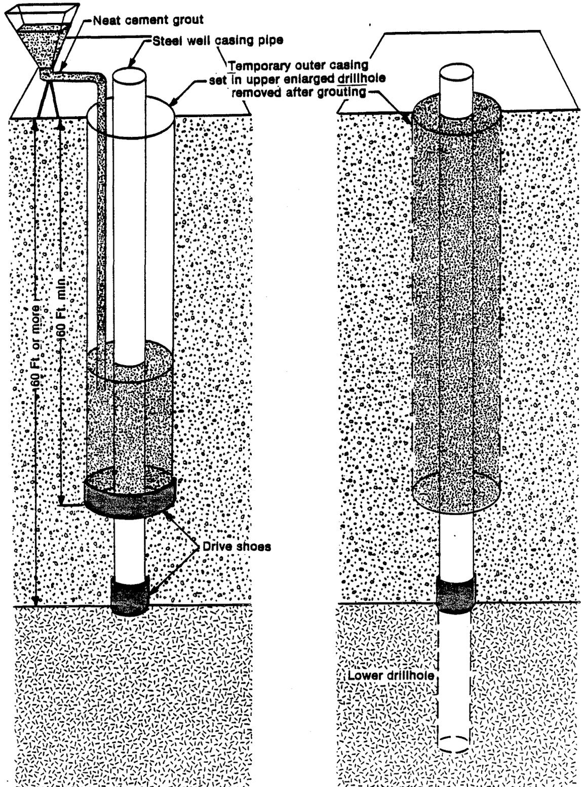
The diameter of the upper enlarged drillhole shall be at least 3 inches larger than the outside diameter of the well casing pipe or well casing pipe couplings, if used. The diameter of the well casing pipe and lower drillhole shall be at least 6 inches.
