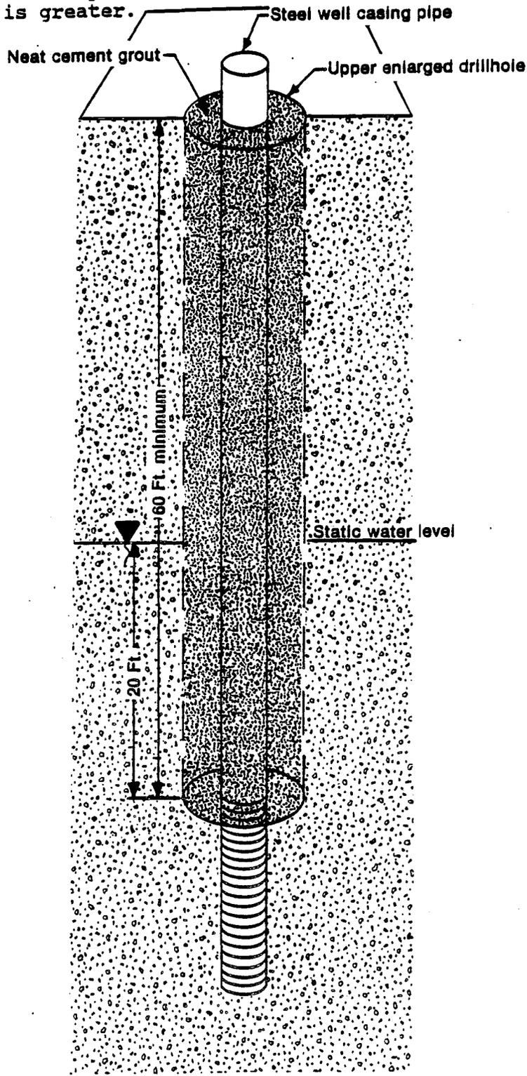
The diameter of the upper enlarged drillhole shall be at least 3 inches larger than the outside diameter of the well casing pipe or well casing pipe couplings, if used.
