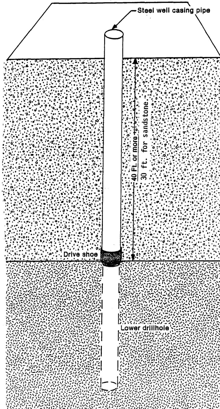
The well casing pipe may be driven from the ground surface.
