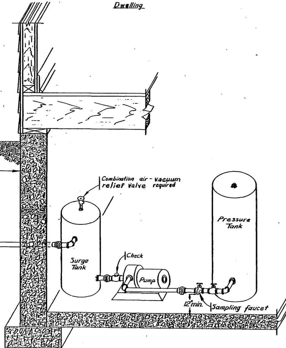
Figure 42. Flowing well installation with a surge tank instead of an overflow piping arrangement.
