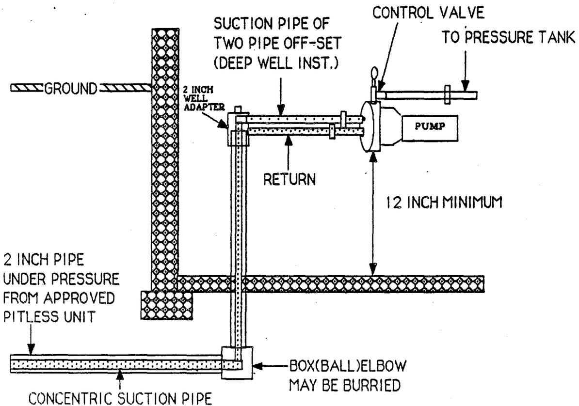
Figure 36b. Offset pump installation discharge piping using a buried box (ball) elbow.
