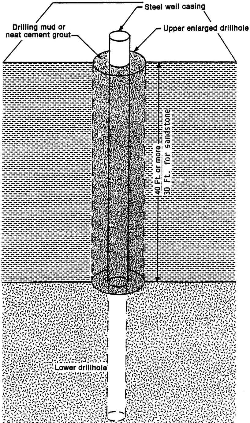
The upper enlarged drillhole shall be at least 2 inches larger in diameter than the nominal well casing pipe diameter for well casing pipe with welded joints. For threaded and coupled well casing pipe, the diameter shall be at least 4 inches larger than the nominal diameter of the well casing pipe. During construction the upper enlarged drillhole shall be maintained at full diameter by circulating drilling mud.
