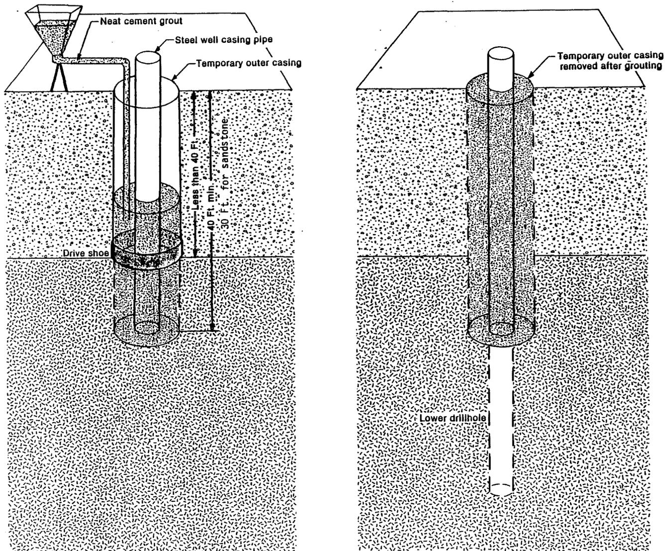
For well casing pipe with welded joints only. For threaded and coupled well casing pipe the diameter shall be at least 4 inches larger than the nominal diameter of the well casing pipe.
