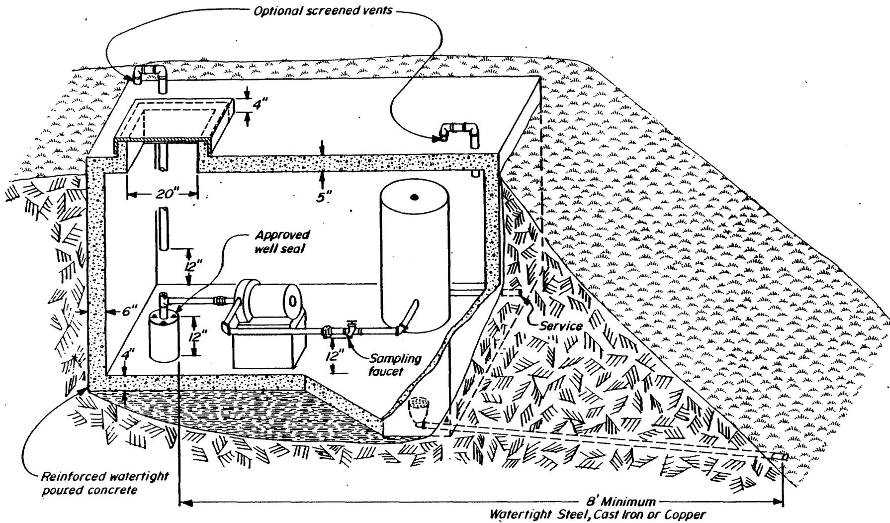
Figure 45. Minimum requirements for approved new well pits.
