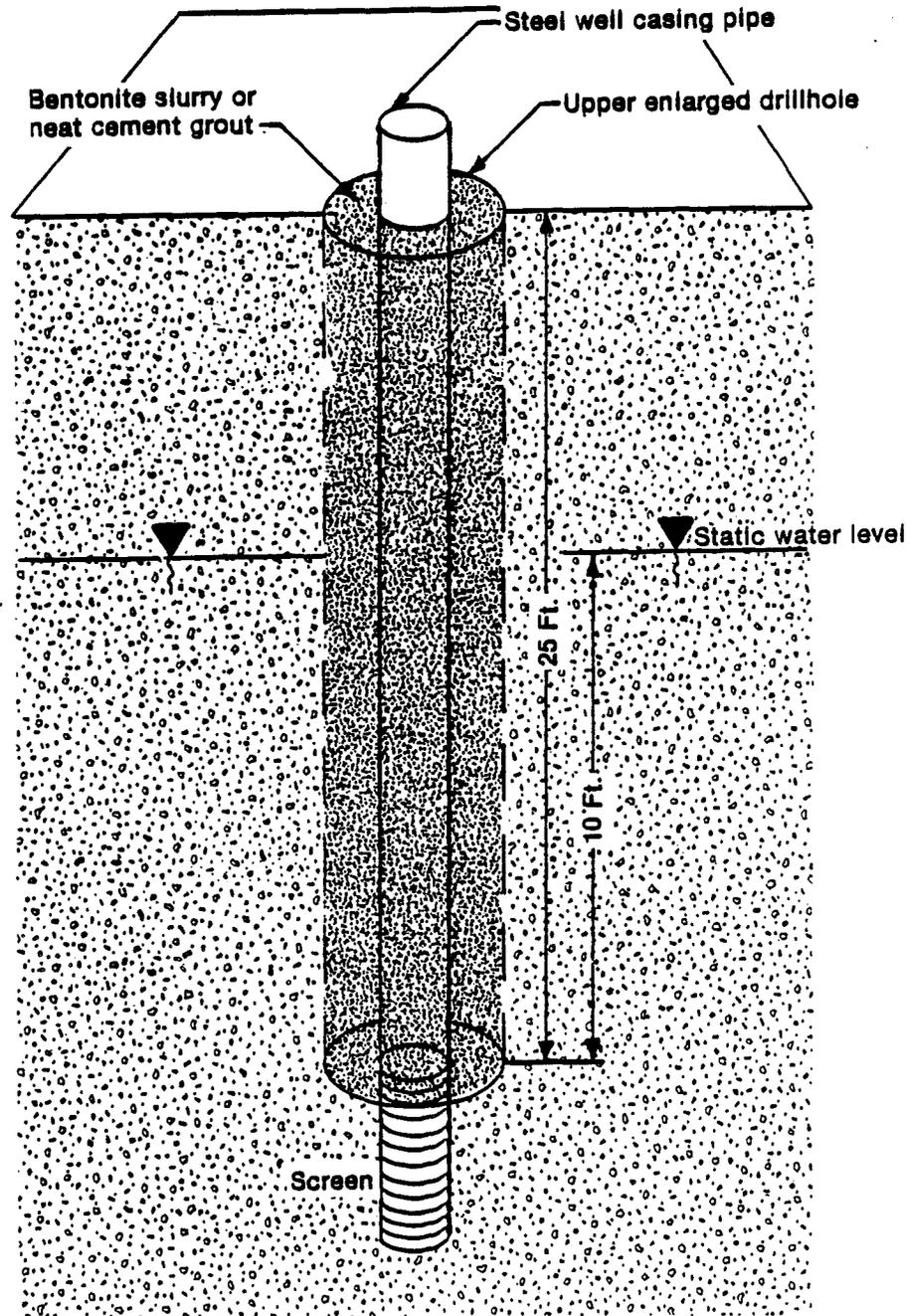
The upper enlarged drillhole shall be at least 2 inches larger in diameter than the nominal well casing pipe diameter for well casing pipe with welded joints. For threaded and coupled well casing pipe, the diameter shall be at least 4 inches larger than the nominal diameter of the well casing pipe. During construction the upper enlarged drillhole shall be maintained at full diameter by circulating drilling mud.
