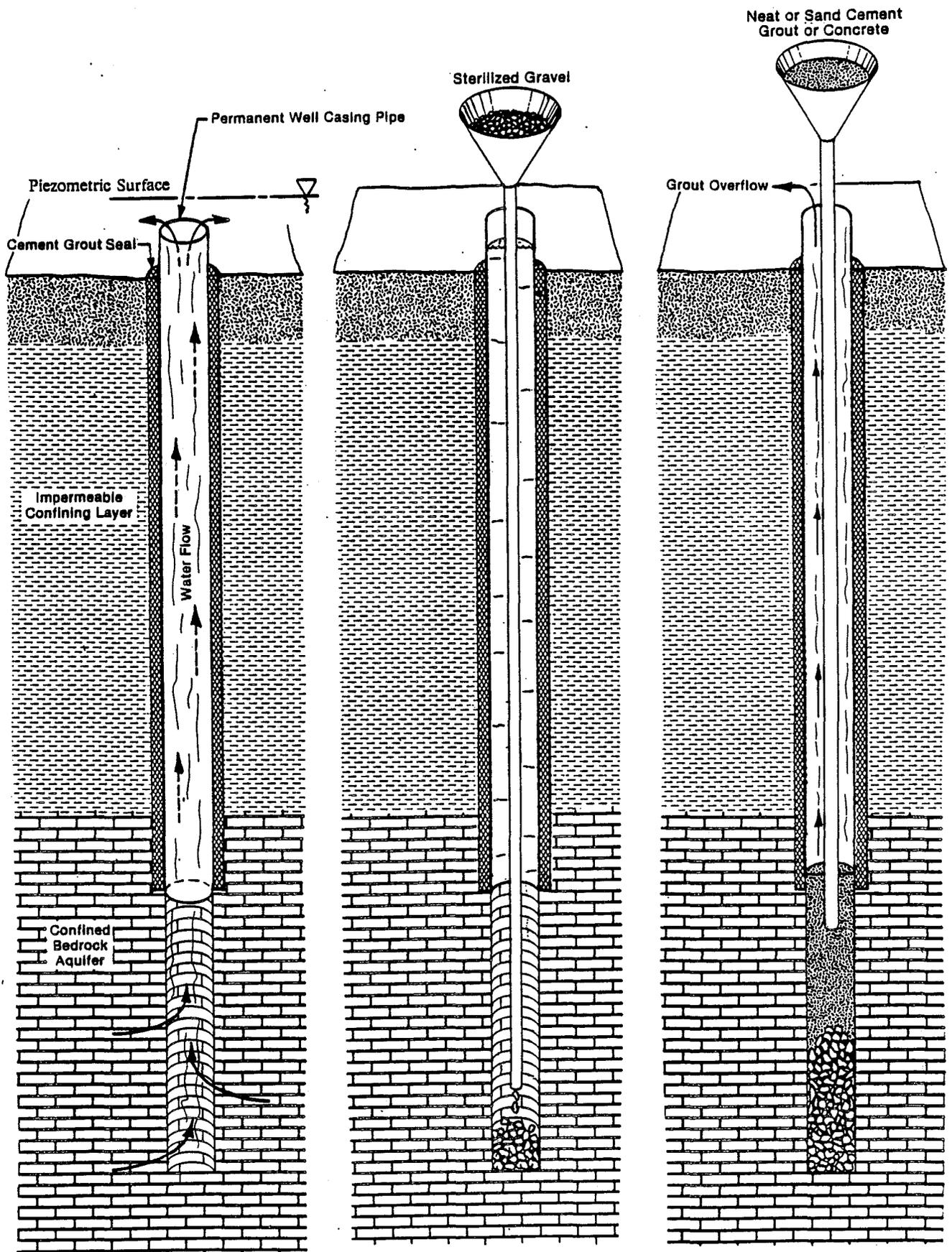
Figure 22. Method for reducing flow in a flowing well by first adding gravel to the bottom before permanently abandoning the well.
