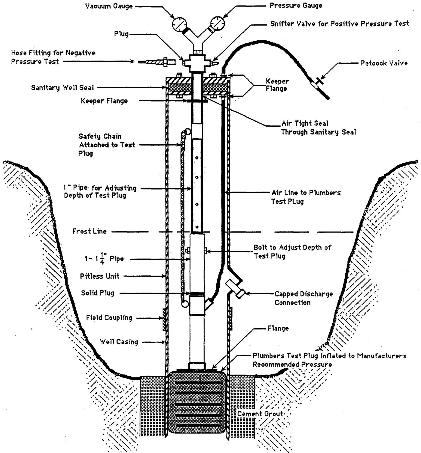
Figure 29. Method for pressure testing a pitless adapter or unit.
