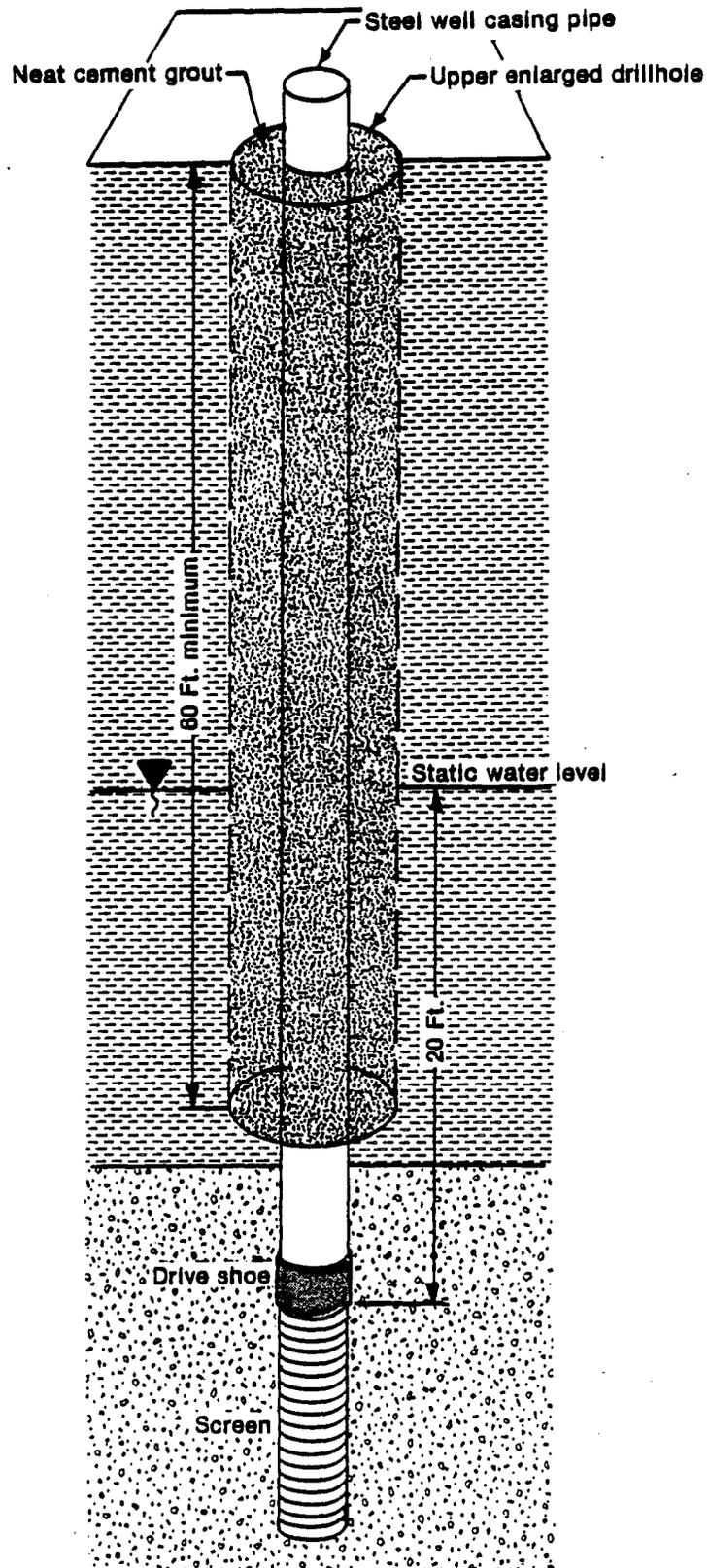
The diameter of the upper enlarged drillhole shall be at least 3 inches larger than the outside diameter of the well casing pipe or well casing pipe couplings, if used.
