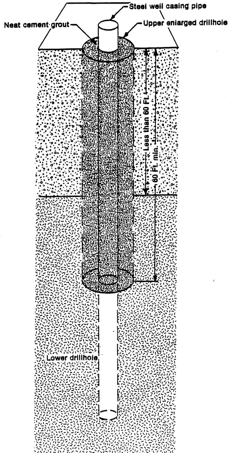
The diameter of the upper enlarged drillhole shall be at least 3 inches larger than the outside diameter of the well casing pipe or well casing pipe couplings, if used. The diameter of the well casing pipe and lower drillhole shall be at least 6 inches.
