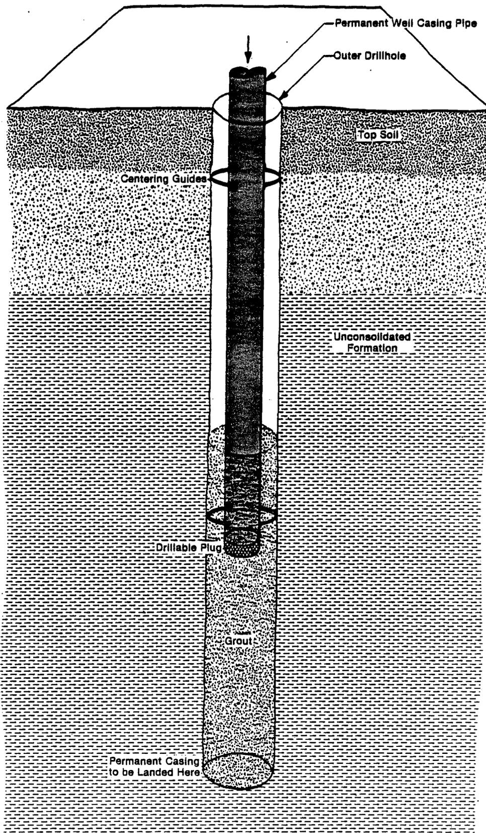
Figure 17. Grout displacement method for neat cement grouting.
