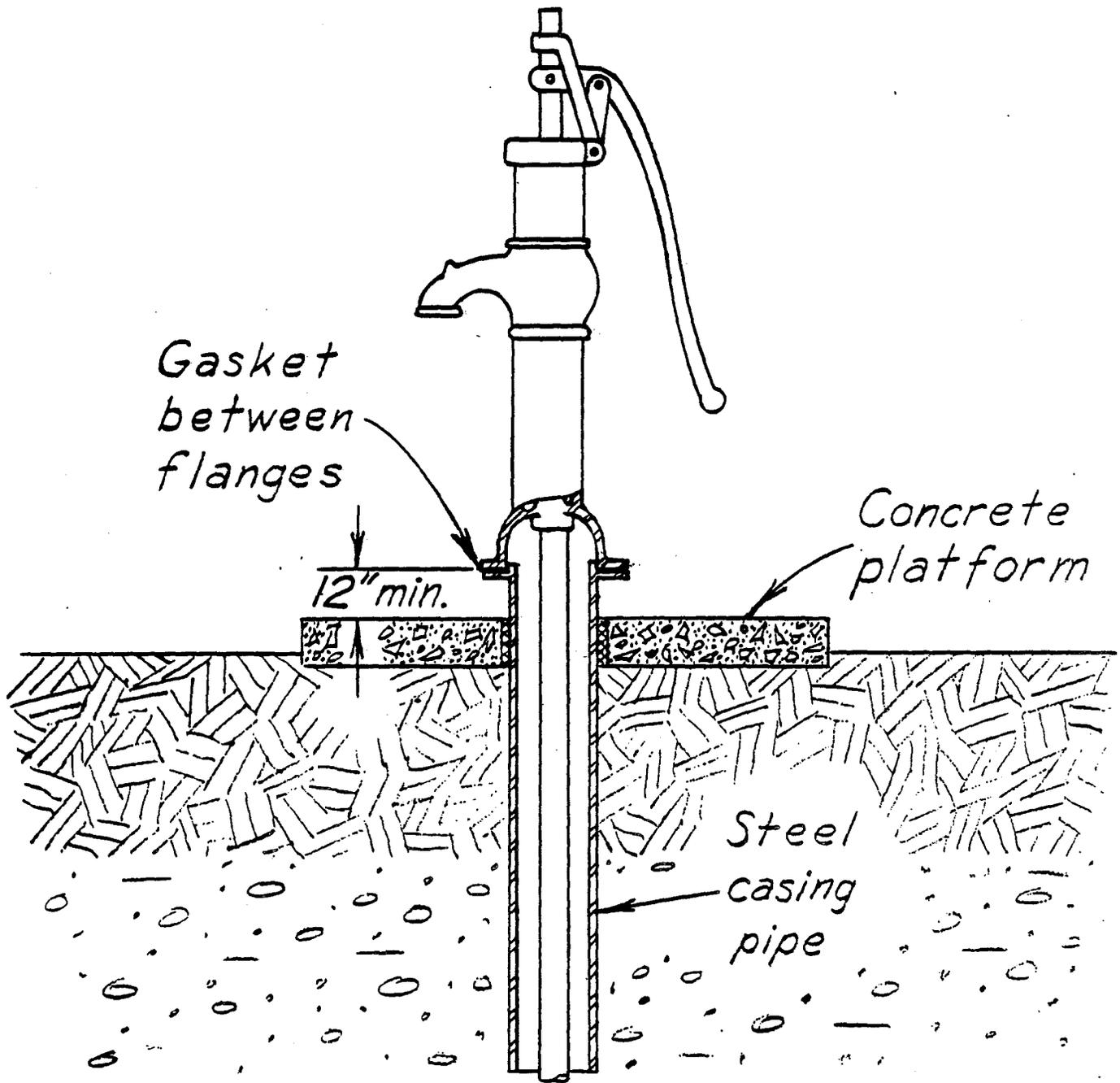
Figure 40. Pump installation for wells with hand pumps.
