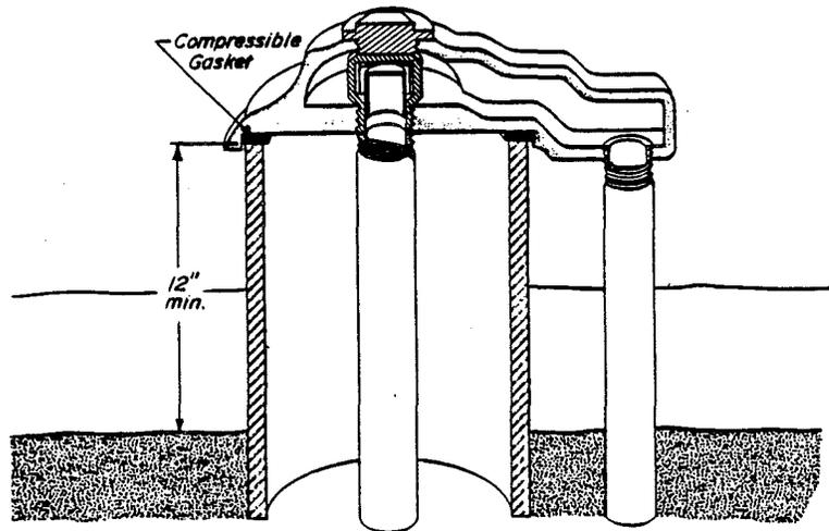
Figure 23. Examples of sanitary well seals.
