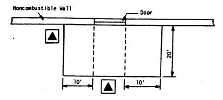
2. Padmounted oil-insulated transformers shall not be located within a zone extending 10 feet outward and 10 feet to either side of an air intake opening. Such transformers may be located within said zone beneath an air intake opening provided there is not less than 25 feet diagonal separation between the transformer and said opening. See Figure PSC 114-317B2.
