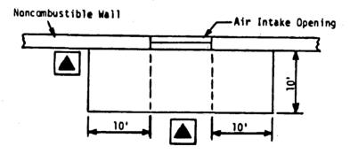
3.a. Padmounted oil-insulated transformers shall not be located within a zone extending 10 feet outward and 3 feet to either side of a building window or opening other than an air intake. See Figure PSC 114-317B3a.
