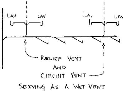
A-82.31 (14) (a) and (b) Sizing vent stacks and stack vents.
