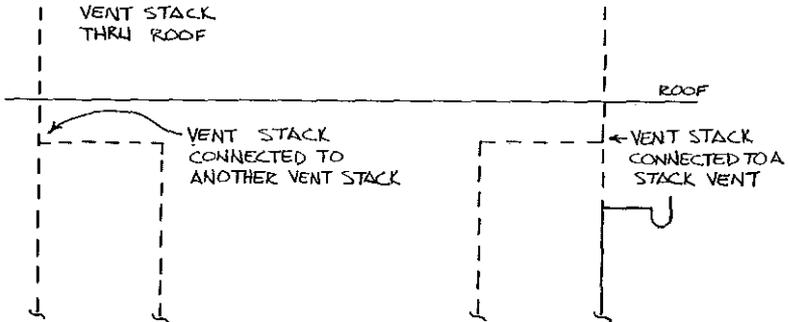
A-82.31 (4) (b) Installation of vent stack and stack vent.
