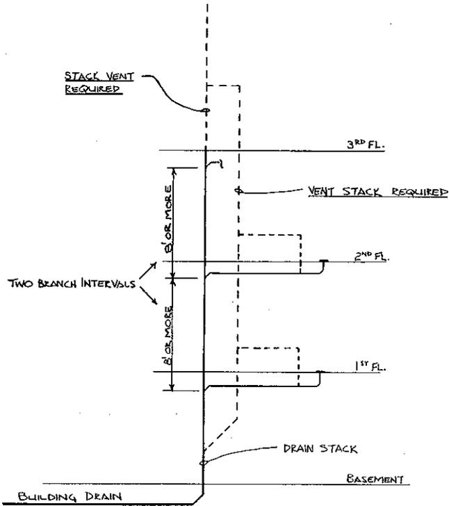
A-82.31 (4) (a) Where a vent stack and stack vent are not required.
