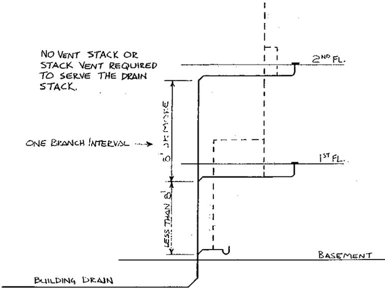
A-82.31 (4) (b) Installation of vent stack and stack vent.
