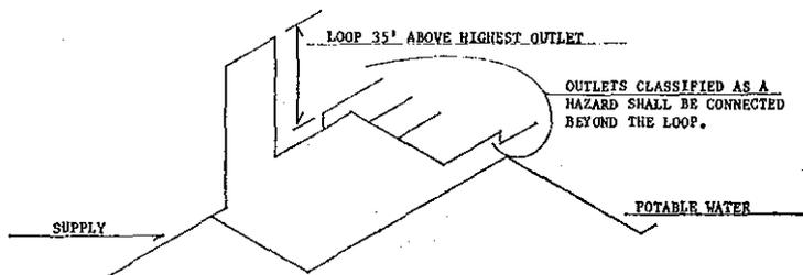
(q) *Turf sprinklers.* Turf sprinkler systems, when connected to a potable water system, shall be installed in accordance with these regulations. Adequate and proper provisions shall be made for control and drainage and to prevent back-siphonage or backflow. Water shall not be turned on to any turf sprinkler system until it has been inspected and approved. Materials used in turf sprinkler systems shall be submitted for evaluation and approval prior to installation.
