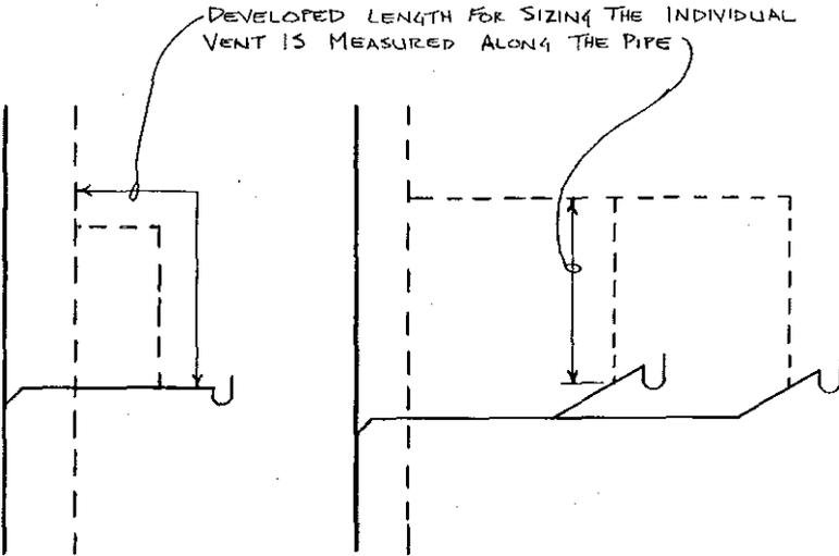
A-82.31 (14) (c) Sizing branch vents serving a wet vent.
