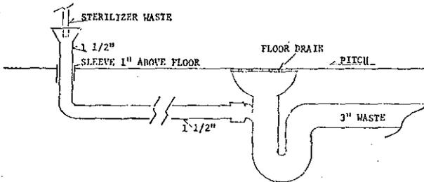
3. **Battery assemblies.** A battery assembly of not more than 3 sterilizer wastes may drain to one trap, provided the trap and waste are sized according to the combined fixture unit rating; the trap is located immediately below one of the indirect waste connections; the developed distance
