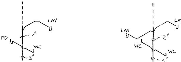
COMMON VENT FOR FLOOR OUTLET FIXTURES
