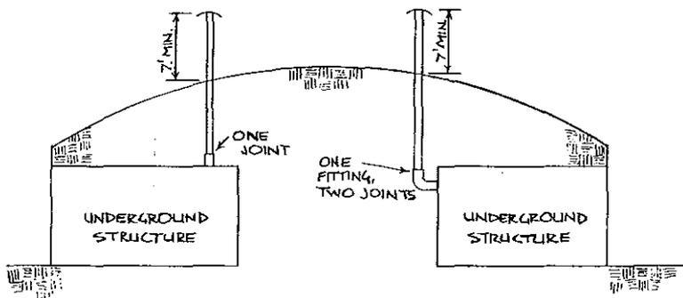
VENT TERMINALS FOR UNDERGROUND STRUCTURES
