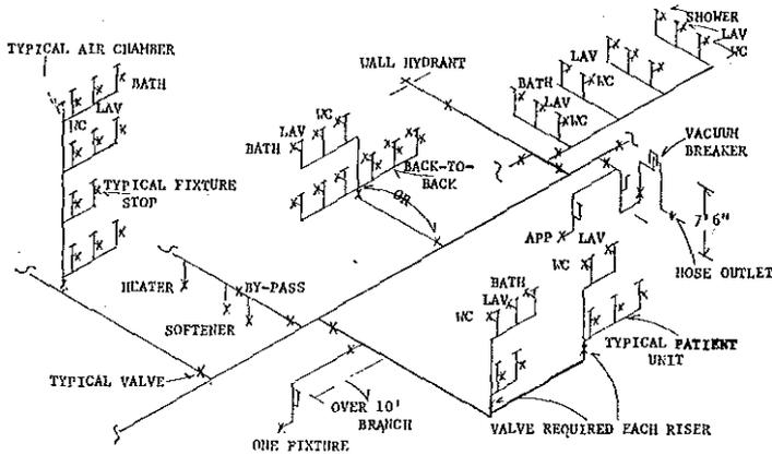
2. Control valves for risers, water heating equipment, water softeners and tank controls shall be in accord with s. ILHR 82.40 (4) (j) 2. b. c. d. and g. Control valve accessibility and design shall be in accord with s. ILHR 82.40 (4) (j) 2. e. and f. See above sketch.
