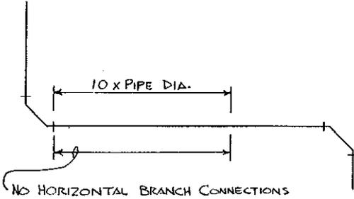
A-82.30 (7) Horizontal branch drain connection at base of a stack.
