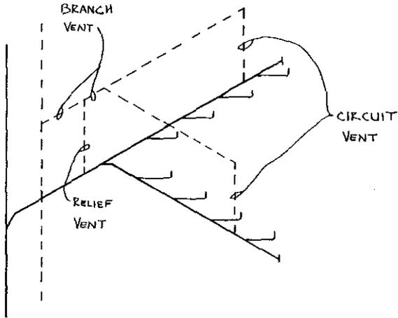
A-82.31 (11) (a) Common vents, vertical drains.
