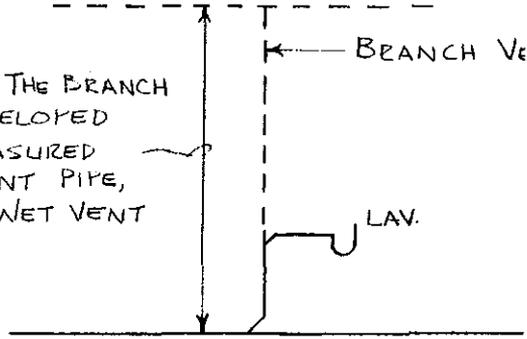
WHEN SIZING THE BRANCH VENT, THE DEVELOPED LENGTH IS MEASURED ALONG THE VENT PIPE, INCLUDING THE WET VENT PORTION.
