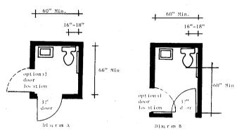
(c) Water closet compartments. Accessible water closet compartments shall be designed in accordance with the minimum design standards as established in Table 52.04-B, or as approved by the department. Sufficient clearance must be maintained to permit the door to the toilet room compartment to open at least 95°.
