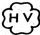
FIG. HG-402 OFFICIAL SYMBOL FOR STAMP TO DENOTE THE AMERICAN SOCIETY OF MECHANICAL ENGINEERS' STANDARD
