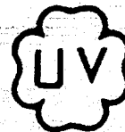
FIG. UG-129 OFFICIAL SYMBOL FOR STAMP TO DENOTE THE AMERICAN SOCIETY OF MECHANICAL ENGINEERS' STANDARD
