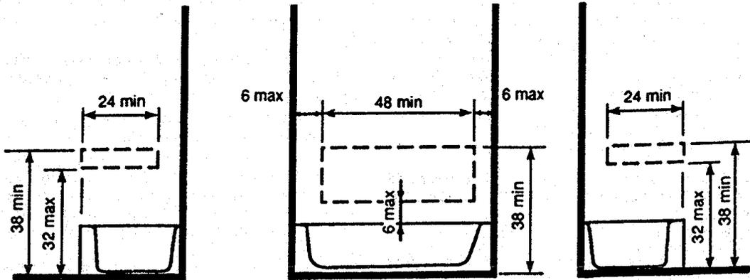
NOTE: The areas outlined in dashed lines represent locations for future installation of grab bars for typical fixture configurations.
