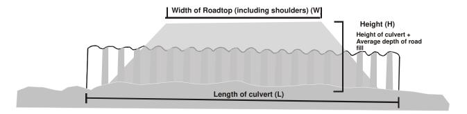
Determining the length of a culvert:
