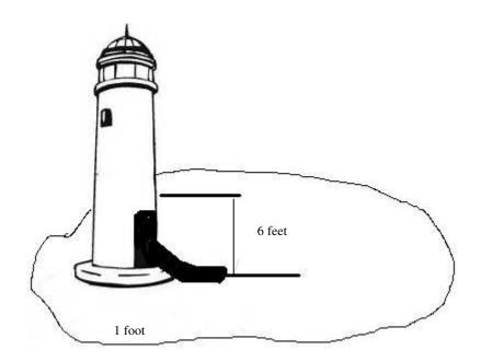
In the drawing above, the obstructed area between the water level to height of 6 feet is 3 square feet. This obstruction would be permitted in a wading pool without a lifeguard plan.
