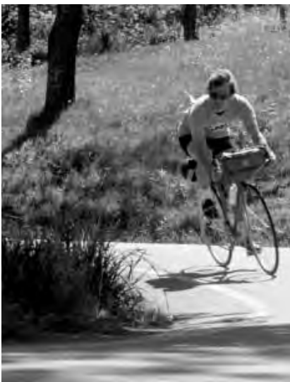
Figure 4-21: A bicyclist entering a curve. Note inside pedal is up in preparation for turning.
