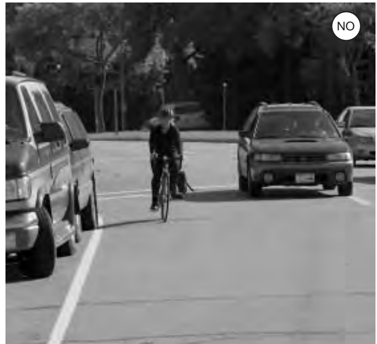
Figure 2-27: Narrowing the parking lane by adding a white line will not necessarily create extra space for bicyclists.
