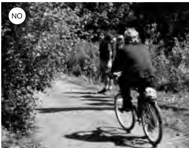
Figure 4-31: Overhanging bushes on the inside of this curve reduce sight distance and narrow the path.
