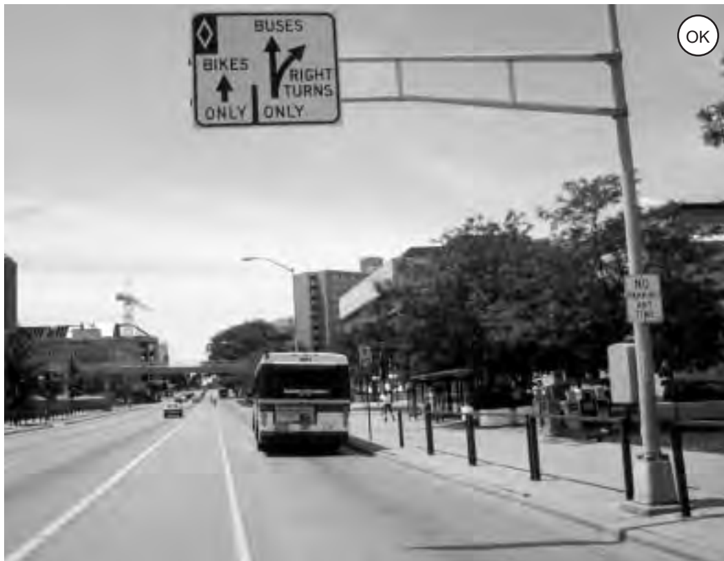
Figure 3-19: A well-used bicycle lane on a busy bus route puts the bicyclists to the left of the buses and right-turning motor vehicles.
