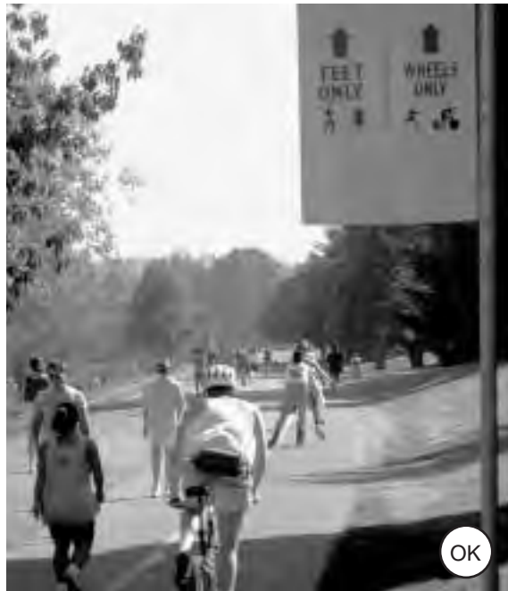
Figure 4-139: One common way to separate bicycles and pedestrians on a shared-use path. Stripes only work well with relatively low pedestrian and/or bicycle volumes. For more on this, see Section 4.14.1.
