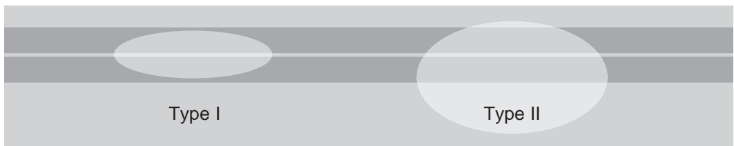
Figure 4-52: Type II horizontal lamps provide more light than is necessary.
