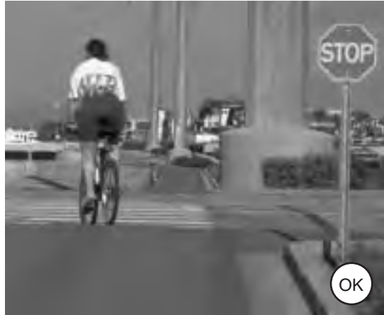
Figure 4-62: The intersection of a path and roadway; in this instance, the path has the stop sign
