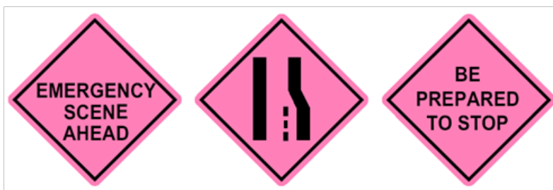
Figure 6.2 - Examples of TIMA Advance Warning Signs
