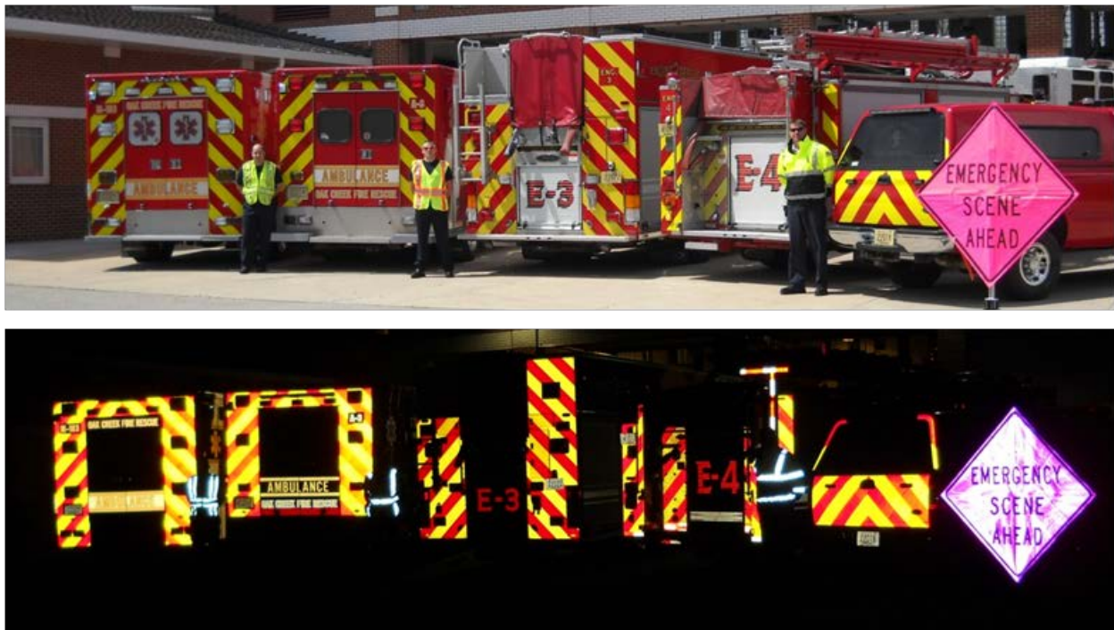
Figure 4.2 - Emergency Vehicles with Retroreflective Chevron Striping (Source: City of Oak Creek Fire Department)
