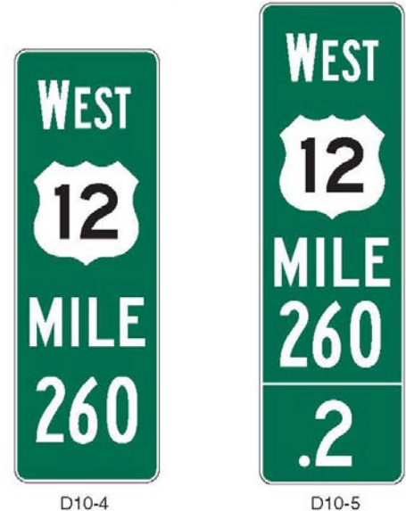
Figure 2H-4. Enhanced Reference Location Signs
