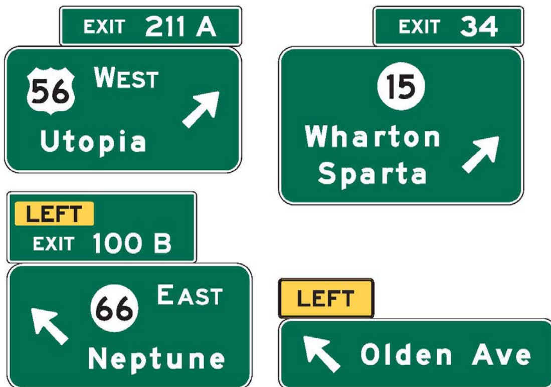
Figure 2E-26. Examples of Interchange Exit Direction Signs
