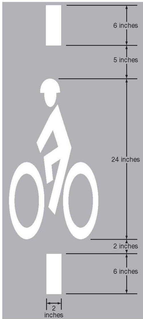
Figure 9C-7. Bicycle Detector Pavement Marking
