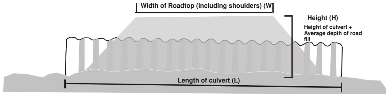
Determining the length of a culvert:
