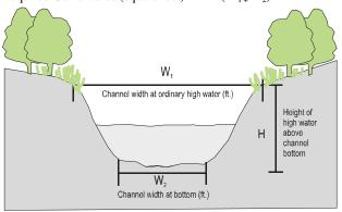
(2) CULVERT SIZING. Once the required culvert area has been determined, the applicant can identify the proper culvert size by
