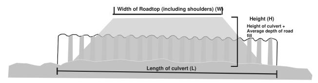
Determining the length of a culvert:
