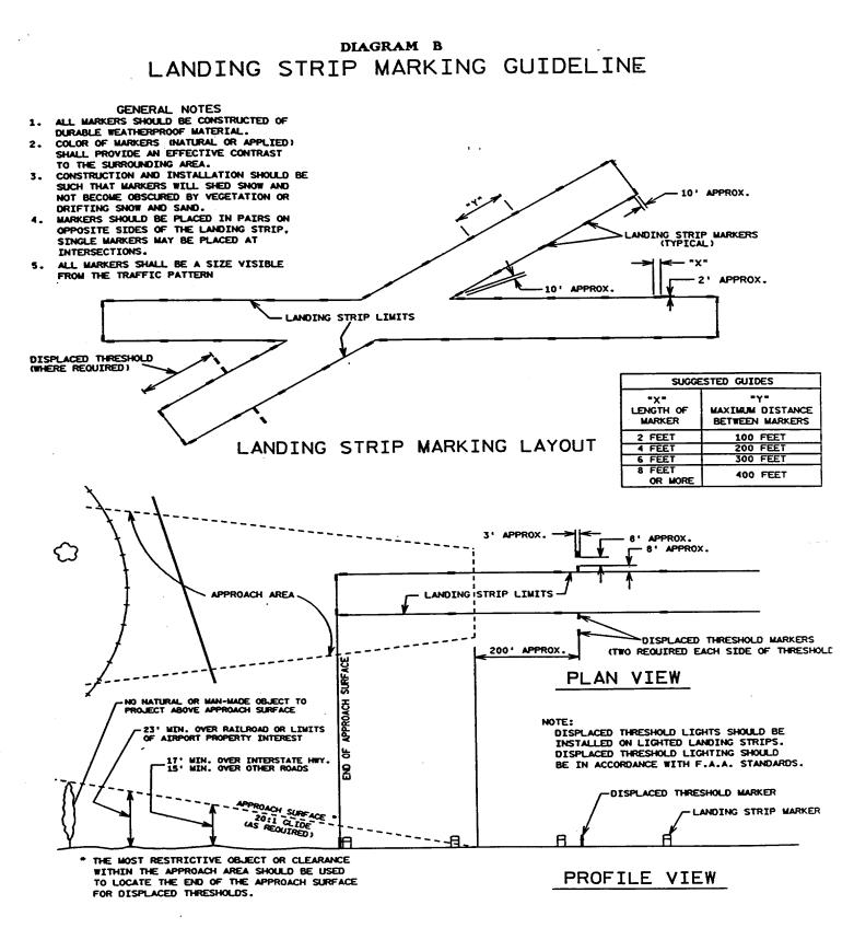
DISPLACED THRESHOLD MARKER LAYOUT
