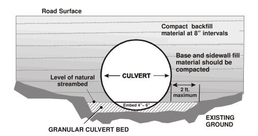
11. Dredging under s. 30.20 (1g) (b) 1., Stats., and deposition of sand, gravel or stone on the stream bed under s. 30.12 (1g) (a), Stats., may be associated with the replacement of a culvert provided dredging is limited to the volume necessary to bury the culvert as required in subd. 5. and the deposit is limited to the area immediately underneath or within 2 feet of the culvert.
