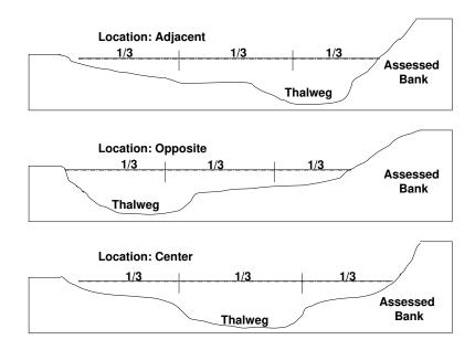
(3) BANK EDGE RECESSION MEASUREMENTS. Methods of measuring bank edge recession shall include all of the following: establishment of a physical measurement reference line between at least 2 headstakes; date-imbedded photographs showing the initial installation of the reference line and headstakes; reference distance measures to the bank lip shall be reported on department supplied forms; and time between separate measurements shall equal or exceed 3 months during the open-water season.
