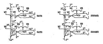
(c) Other fixtures. A horizontal soil or waste pipe to which 2 and not more than 8 like fixtures are connected may be vented by a circuit
