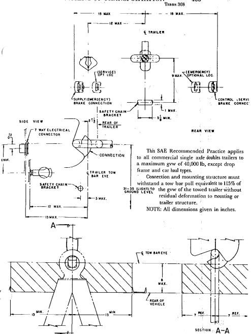
Clearance space shown must extend 7 in, above and 7 in, below the horizontal centerline of the drawbar eye as shown in Section A-A.
