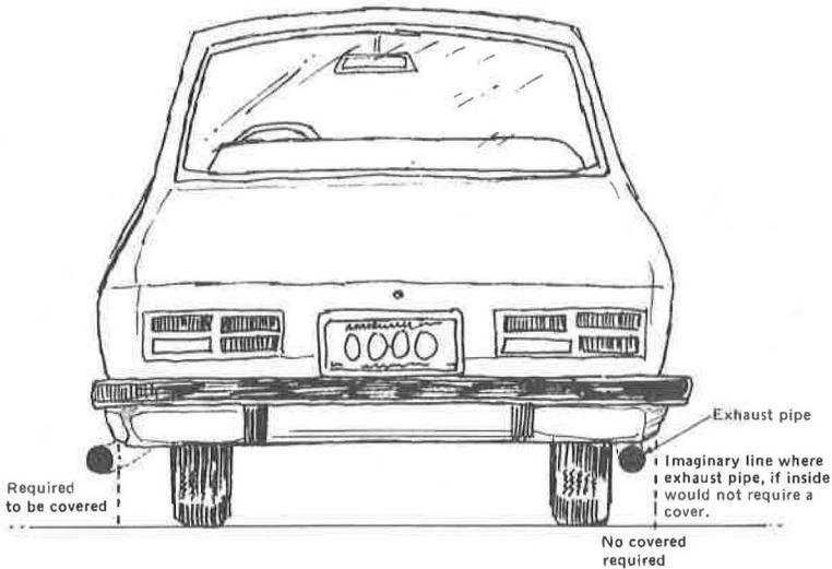
(a) The muffler or any part of the exhaust system has been repaired by an inadequate patch, is not adequate for discharging fumes or non-rigid type tubing is used except in the case of motor driven cycles, road tractors, truck tractors or trucks over 10,000 pounds GVW where the connection is outside the cab line.
