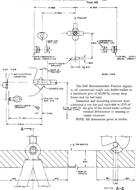
Clearance space shown must extend 7 in. above and 7 in. below the horizontal centerline of the drawbar eye as shown in Section A-A.
