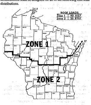
(4) ROOF LOADS. Roof structural members subject to snow accumulation shall be designed for all of the following roof load
